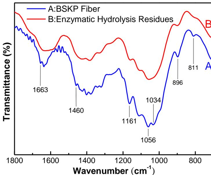
Fig. 5. FTIR spectra patterns of the untreated pulp and enzymatic hydrolysis residues
