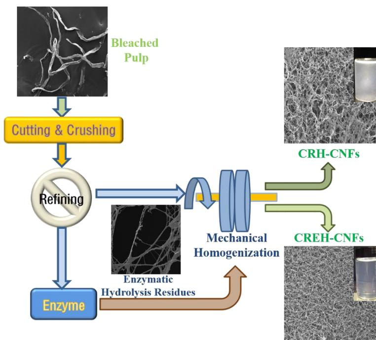
Fig. 1. Schematic process flow diagram of experiments
