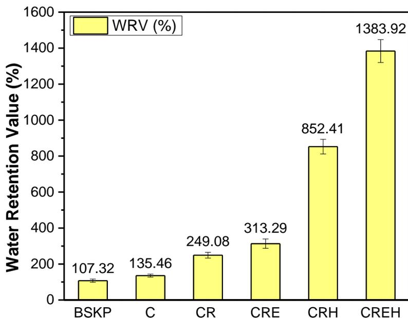
Fig. 3. Water retention value (WRV) of cellulose fiber from different conditions
