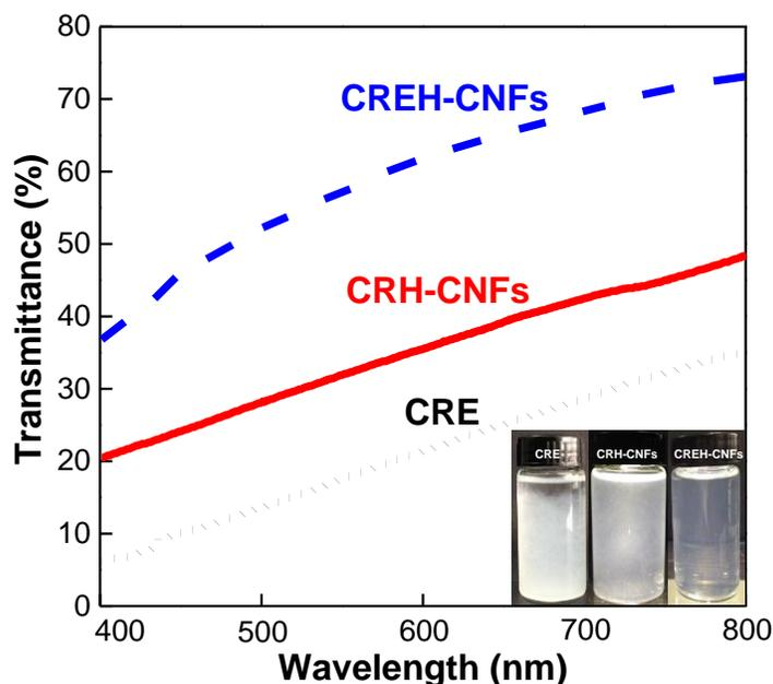
Fig. 6. UV-vis light transmittance of suspension from CRE, CRH-CNFs, and CREH-CNFs
