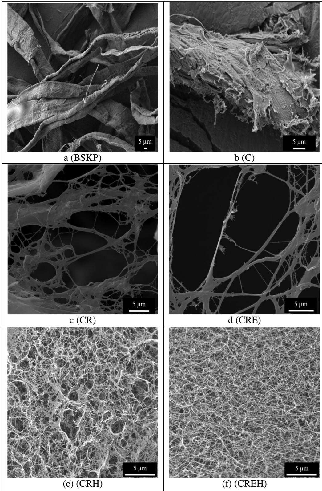
**Fig. 2.** SEM images of BSKP fibers under different conditions. (a) - (f) represent BSKP, C, CR, CRE, CRH, and CREH, respectively. The scale bar is 5 μm.
