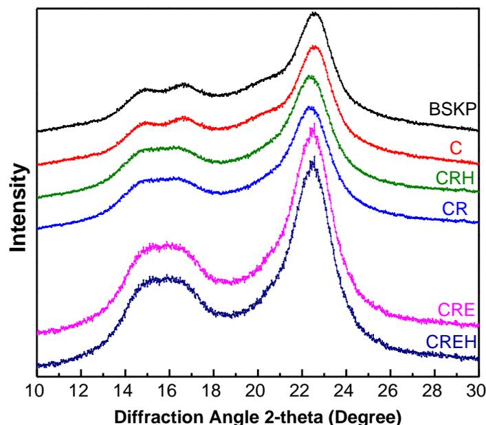
Fig. 4. XRD patterns for BSKP and different cellulose fibers
