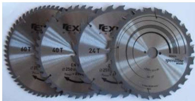
Fig. 2. Saw blades used, from left to right: 24, 40, and 60 teeth; 24 teeth and a chip limiter
