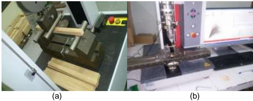
Fig. 2. (a) Standard-size bending test sample and test setup; (b) micro-size bending test sample and test setup
