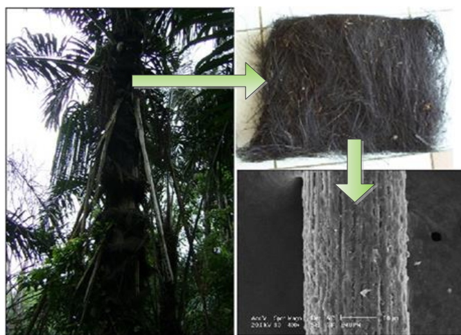
Fig. 4. Sugar palm tree, its fibre, and SEM image of single fibre (Bachtiar et al. 2008; Ishak et al. 2013)
