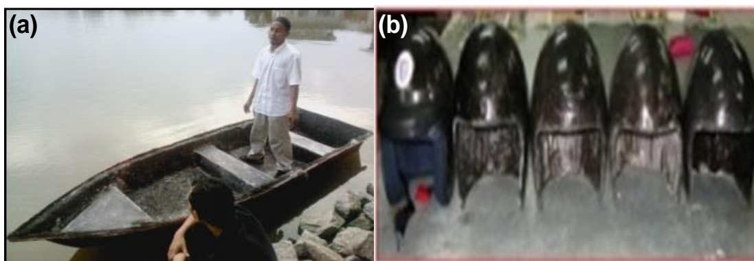
Fig. 8. SPF product development (a) small boat and (b) safety helmet (Zaid 2009; Misri et al. 2010)
