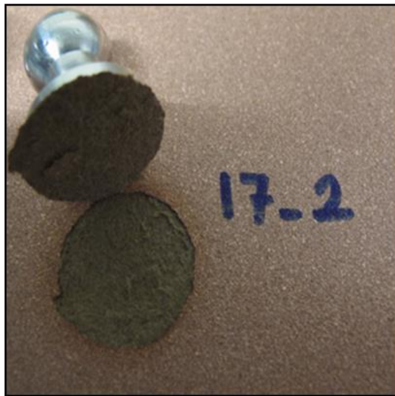
Fig. 4. Image of an MDF sample after the pull-off adhesion test
