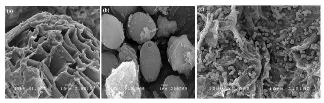
**Fig. 4.**Scanning electron micrographs of wCTF: a and b) before and c) after fermentation. a) The porous structure of the wCTF with attached residual yeast cells (1000X magnification), b) the budding scar of the attached cell (10,000X magnification), andc) the increased cell number attached to wCTF after fermentation (1000X magnification). Images are representative of at minimum of 3 fields of view per sample and 2 independent samples
