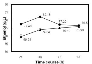
**Fig. 3.** Ethanol production by *S. cerevisiae* G6-2-2 from molasses medium (20% (w/v) sugar) as ( $\blacktriangle$ ) free cells or (•) wCTF-adsorbed cells. Fermentation wasat 40 °C for 48 h. Data represent the mean ± standard deviation (1), derived from 3 independent replicates
