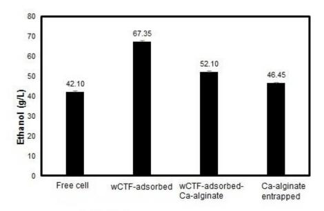
**Fig. 2.** Effect of the immobilization method on the ethanol production. Free (suspension) *S. cerevisiae* G6-2-2 cells  $(1.31 \times 10^{10})$  or those immobilized onto 1.2 g (dry weight) of wCTF and calcium alginate entrapment were employed for the fermentation of 15% (w/v) glucose-containing medium at 40 °C for 48 h. Data represent the mean ± standard deviation (0.6), derived from 3 independent replicates
