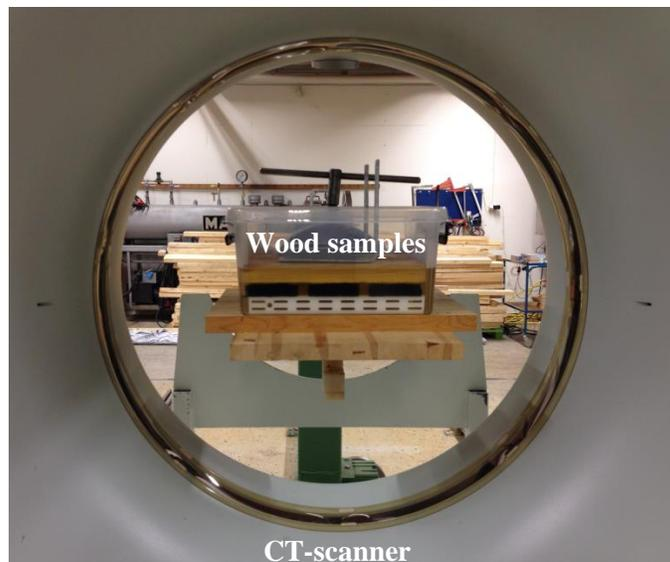
**Fig. 2.** Set of three samples positioned inside the CT-scanner field of view
