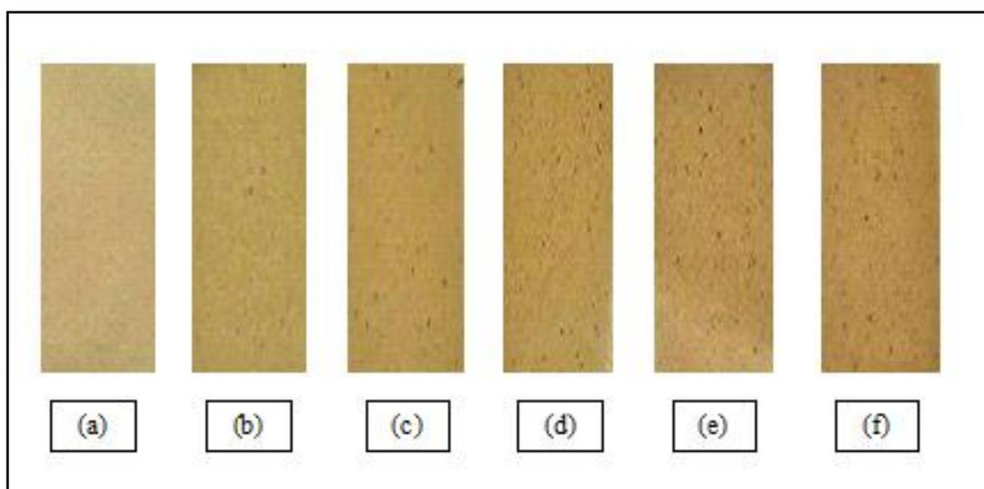
**Fig. 1.** Samples of the composite films with varying EFB pulp fiber loadings: (a) 0%, (b) 10%, (c) 20%, (d) 30%, (e) 40%, and (f) 50%
