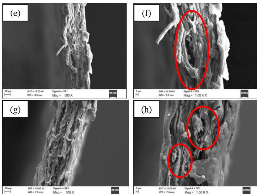
**Fig. 3.** SEM micrograph of fracture surfaces of the seaweed films with varying EFB pulp content. (a) 0%, (c) 10%, (e) 30%, and (g) 50% at 500 times magnification. (b) 0%, (d) 10%, (f) 30%, and (h) 50% at 1000 times magnification. The red circles in (c), (f), and (h) indicate fiber pull-out and breakage.
