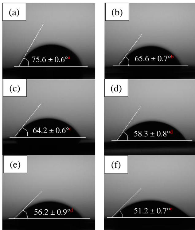
**Fig. 4.** Sessile drops for static water contact angle of the seaweed films with varying EFB pulp content: (a) 0%, (b) 10%, (c) 20%, (d) 30%, (e) 40%, and (f) 50% (<sup>a, b, c, d, e</sup> Values along each row with the same capital letter are not significantly ( $p > 0.05$ ) different as analyzed by Tukey's Test)
