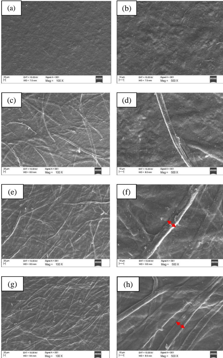
**Fig. 2.** SEM micrographs of the seaweed films with varying EFB pulp concentrations. (a) 0%, (c) 10%, (e) 30%, and (g) 50% at 100 times magnification. (b) 0%, (d) 10%, (f) 30%, and (h) 50% at 500 times magnification. The red arrows in (f) and (h) indicate the average diameter of fiber.
