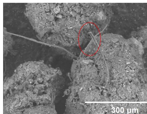
**Fig. 4.** Scanning electron micrograph of bamboo paper sludge
