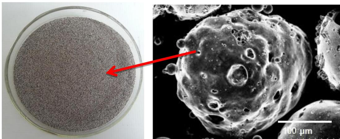
**Fig. 2.** Scanning electron micrograph of fly ash floating beads
