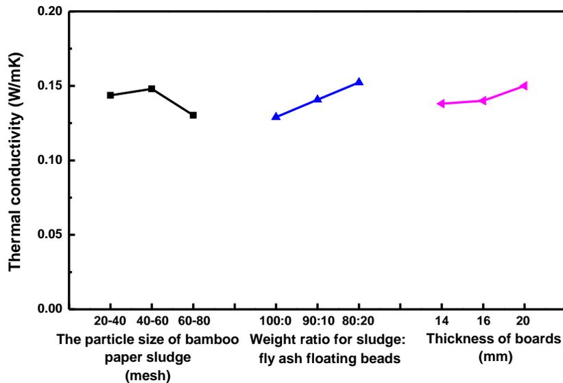
Fig. 7. Effects of different factors on thermal conductivity
