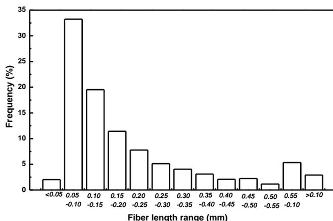
**Fig. 3.** Length distributions of fibers in bamboo paper secondary sludge
