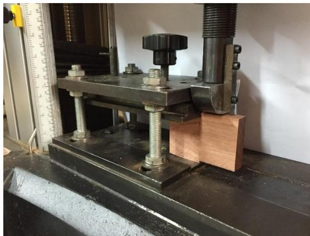
**Fig. 2.** Shear strength test setup
