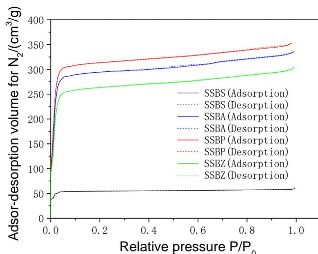
Fig. 5. Adsorption-desorption curves for  $N_2$  of the biochars from sunflower straw
