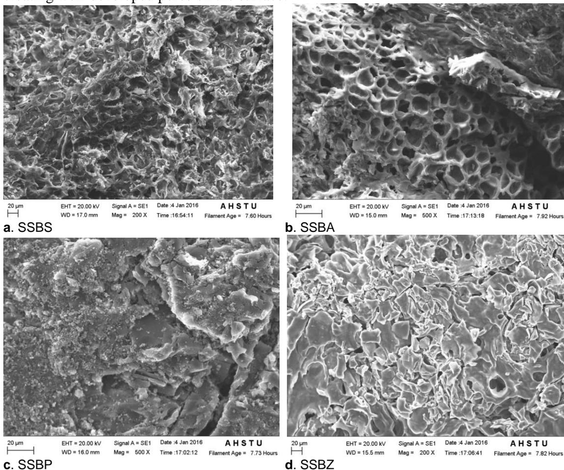
Fig. 3. The SEM morphologies of biomass carbon/activated carbon with four methods
