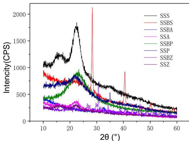
Fig. 2. X-ray diffraction patterns of the biochars from sunflower straw
