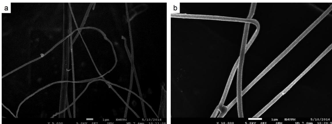
**Fig. 7.** Microfibrillated cellulose produced from 6% (w/v) OPMF-cellulose dissolved in ([EMIM]Cl), ([C<sub>10</sub>MIM][Cl]) and DMF under (a) 5,000x and (b) 10,000x magnifications
