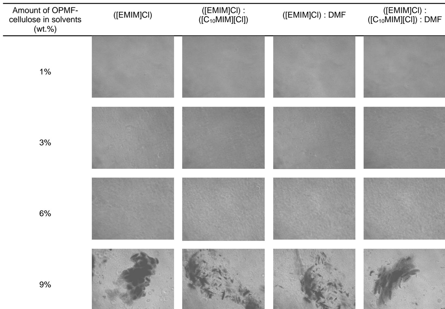
**Fig. 3.** Dissolution of OPMF-cellulose in different ionic liquid solutions as observed under light microscope (40x magnification).
