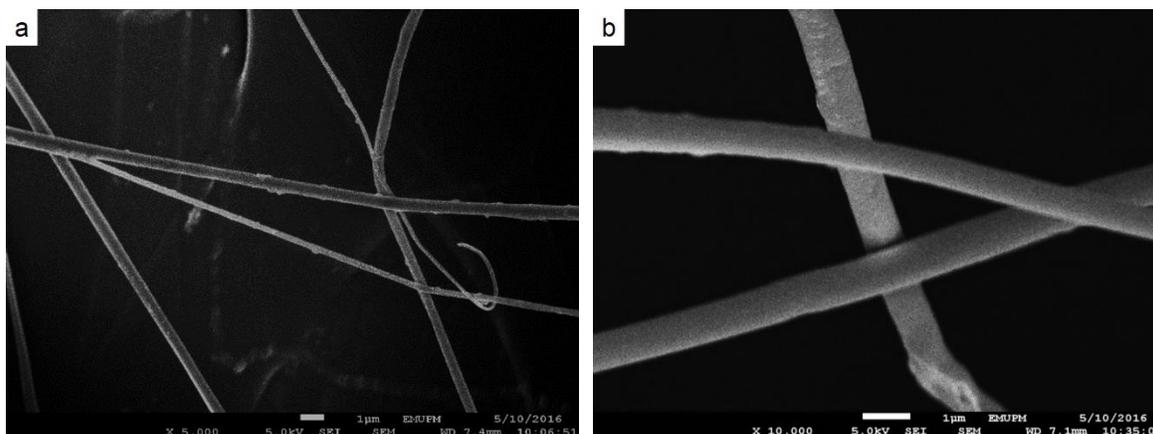
**Fig. 6.** Microfibrillated cellulose produced from 6% (w/v) OPMF-cellulose dissolved in ([EMIM]Cl) and DMF under (a) 5,000x and (b) 10,000x magnifications
