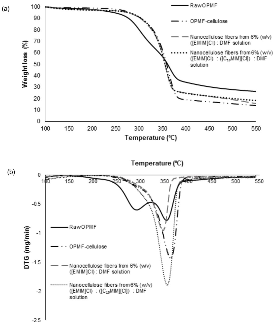
**Fig. 2.** (a) TGA and (b) DTG thermograms of raw OPMF, OPMF-cellulose, MF from 6% (w/v) of ([EMIM]Cl):DMF solution and ([EMIM]Cl):([C<sub>10</sub>MIM][Cl]):DMF solution
