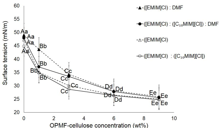
**Fig. 5.** The effect of DMF addition on the surface tension of the OPMF-cellulose solutions at different cellulose concentrations. Capital letters indicate differences ( $P < 0.05$ ) for OPMF-cellulose concentration, while small letters indicate differences ( $P < 0.05$ ) for ionic liquid formulations. All data are means of 3 replicates  $\pm$  S.D. (Different alphabets indicate significant difference, and *vice-versa*).
