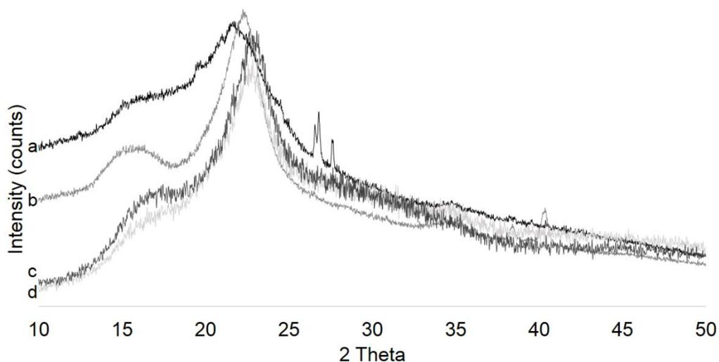
**Fig. 1.** X-ray diffraction patterns of (a) raw OPMF, (b) OPMF-cellulose, and MF from (c) 6% (w/v) ([EMIM]Cl):([C<sub>10</sub>MIM][Cl]):DMF and (d) 6% (w/v) ([EMIM]Cl):DMF solutions
