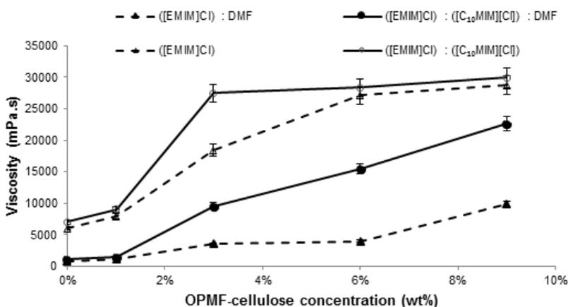
**Fig. 4.** The effect of DMF addition on the viscosity of the OPMF-cellulose solutions at different cellulose concentrations
