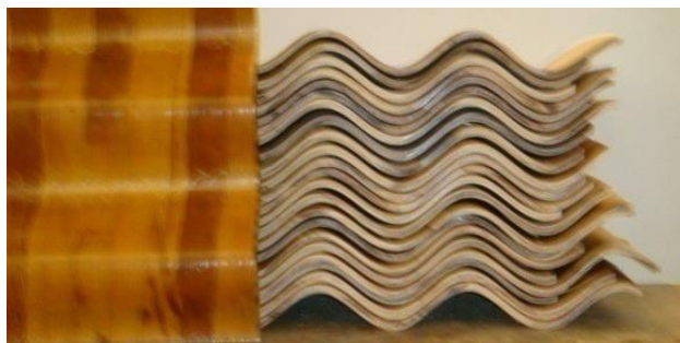
Fig. 9. 9.5 mm thick, sine-wave corrugated panels made of mixed hardwood side-clippings
