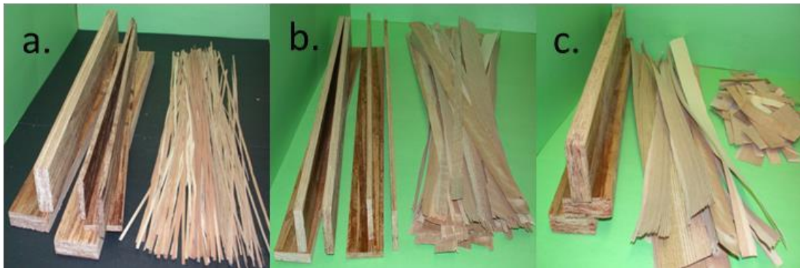
Fig. 3. Variety of structural composites made from veneer clippings: (a) single-layer beams and panels from shredded side-clippings; (b) structural panels from side-clippings; (c) three-layer structural composite with end-clippings in the core
