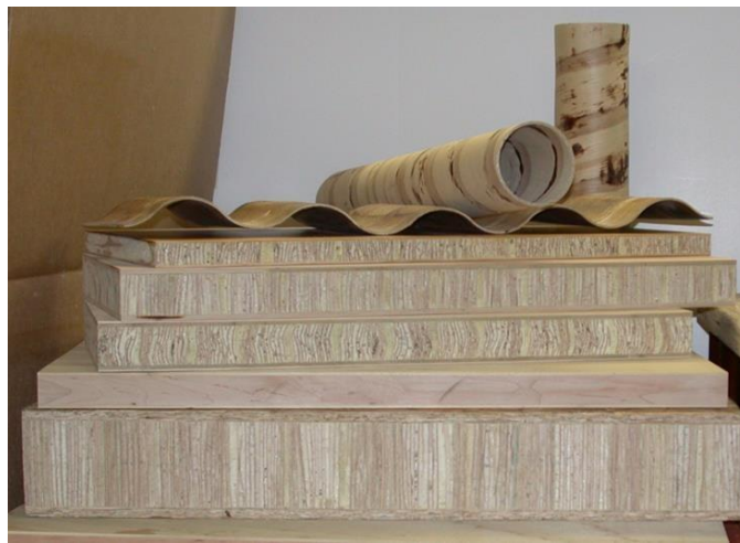
Fig. 2. Variety of panels with PUR – side-clippings core materials and 3-D composites
