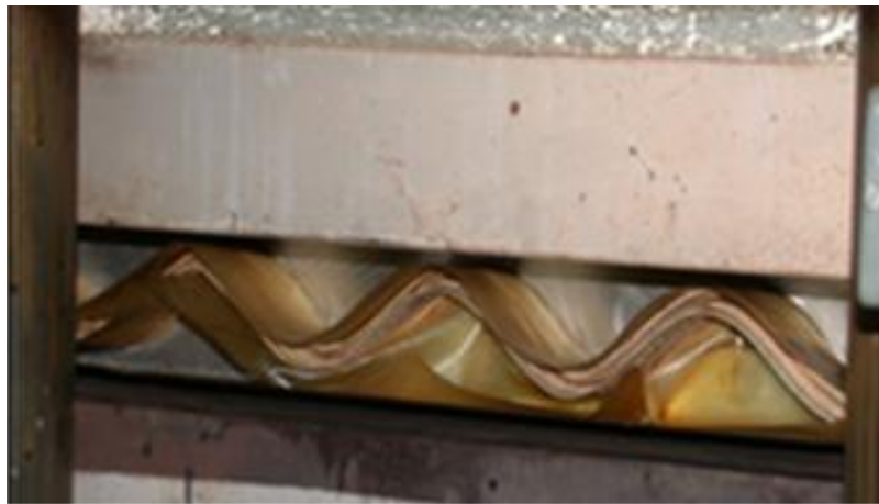
Fig. 5. Sine-wave corrugated panel during the pressing operation
