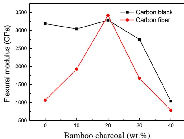
**Fig. 2.** The variation of flexural moduli of the CB and CF composites as a function of bamboo charcoal content
