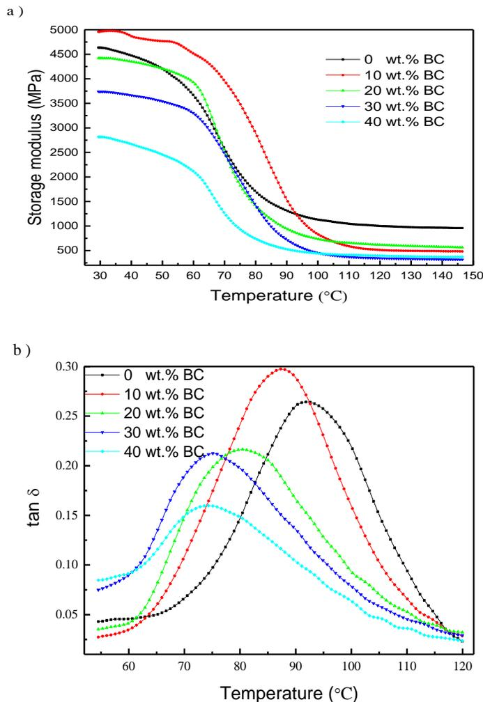
**Fig. 3.** Variation of the storage moduli and loss factor of the CB composite as a function of temperature: a) Storage modulus; b) Loss factor
