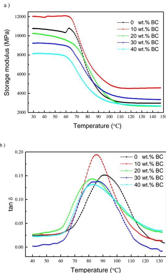
**Fig. 4.** The variation of the storage moduli and loss factor of the CF composite as a function of temperature: a) Storage modulus; b) Loss factor
