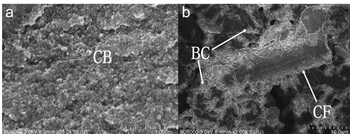
**Fig. 5.** The SEM images of BC composites: a: (8.9 mm × 35.0 k) the CB composites with 10 wt.% BC; b: (8.4 mm × 3.00 k) the CF composites with 10 wt.% BC
