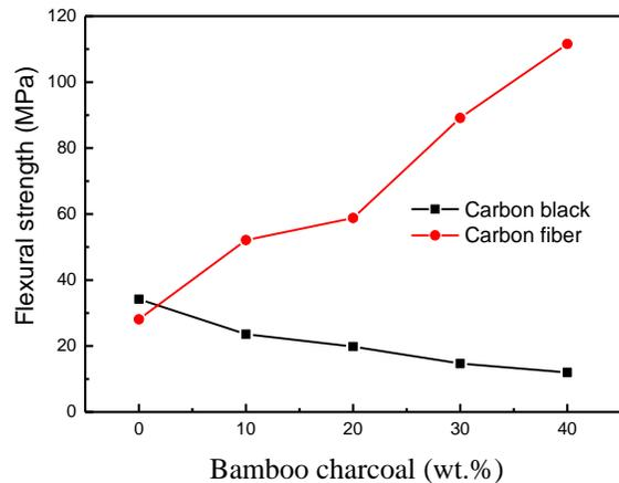
**Fig. 1.** The variation of flexural strengths of the CB and CF composites as a function of bamboo charcoal content
