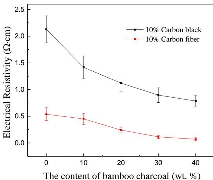
**Fig. 6.** The variation of the electrical resistivity of the CB and CF composites as a function of BC content
