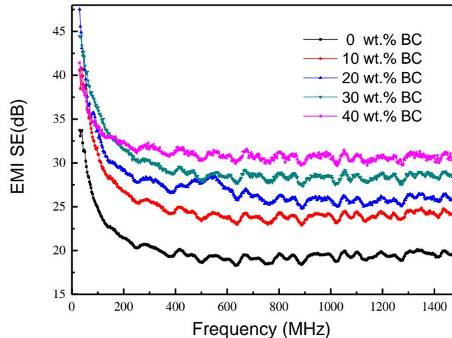
Fig. 7. Variation of EMI SE of the CB composites as a function of frequency
