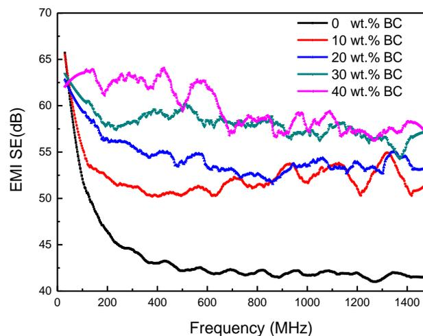
Fig. 8. The variation of EMI SE of the CF composites as a function of frequency
