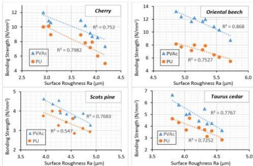
**Fig. 5.** Relationship between bonding strength and surface roughness
