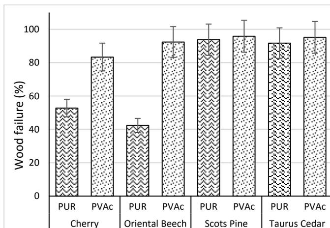
**Fig. 3.** Wood failure percentage of the specimens
