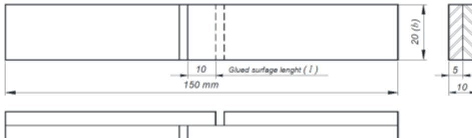
Fig. 1. Dimensions of tensile shear specimen (mm)
