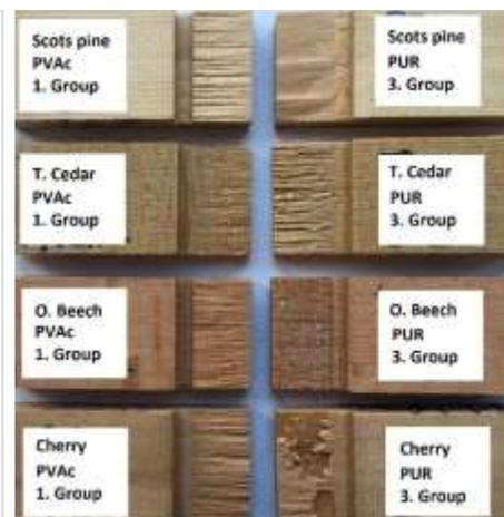
**Fig. 4.** Wood failure
