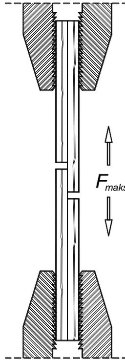
**Fig. 2.** Principle of tensile shear experiment
