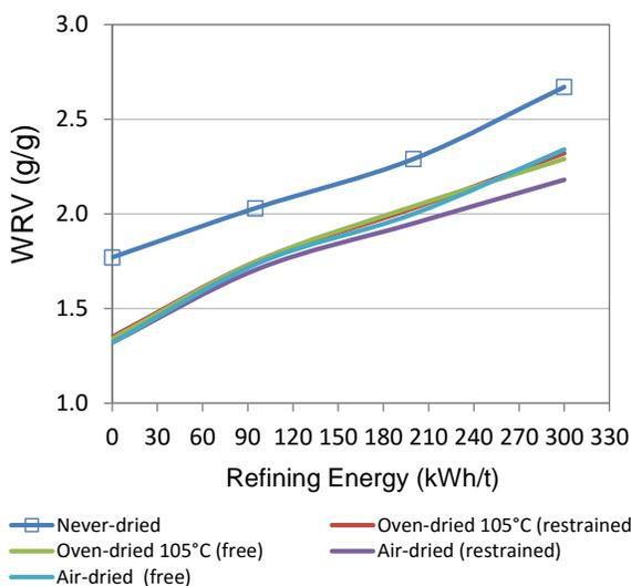
**Fig. 11.** WRV vs. refining energy for pulps refined in Voith Sulzer
