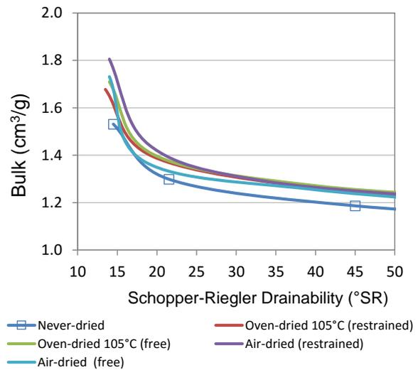
**Fig. 10.** Bulk vs. Schopper-Riegler drainability for pulps refined in Voith Sulzer
