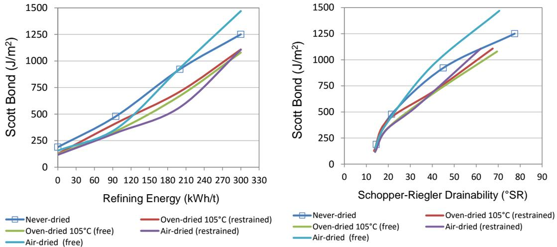
**Fig. 7.** Scott bond vs. refining energy for pulps refined in Voith Sulzer
