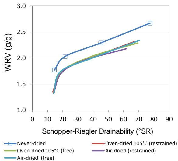
**Fig. 12.** WRV vs. Schopper-Riegler drainability for pulps refined in Voith Sulzer
