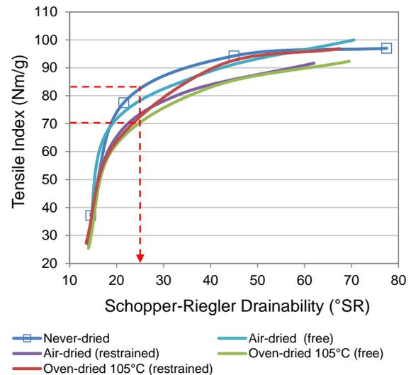
**Fig. 2.** Tensile index vs. Schopper-Riegler drainability for pulps refined in Voith Sulzer
