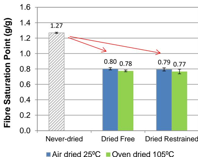
**Fig. 13.** Fiber saturation point for dried and never-dried *Pinus radiata* pulps, including confidence interval at 95%
