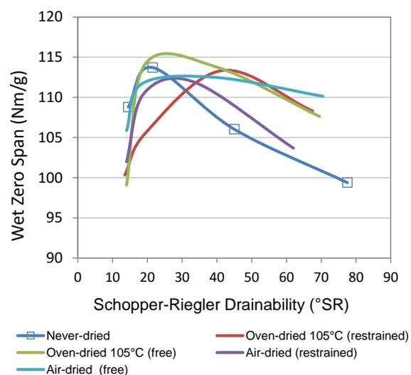
**Fig. 4.** Zero-span vs. Schopper-Riegler drainability for pulps refined in Voith Sulzer
