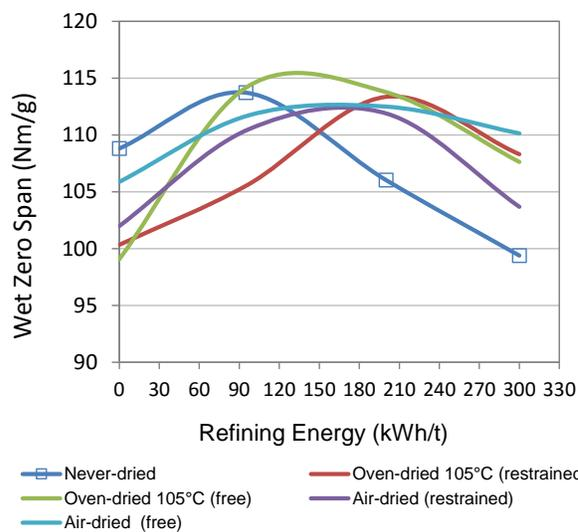
**Fig. 3.** Zero-span vs. refining energy for pulps refined in Voith Sulzer
