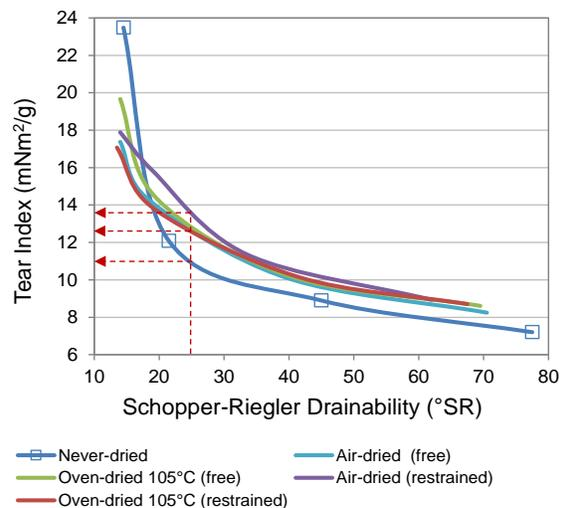
**Fig. 6.** Tear index vs. Schopper-Riegler drainability for pulps refined in Voith Sulzer
