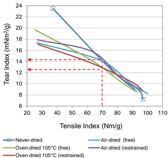
**Fig. 5.** Tear index vs. tensile index for pulps refined in Voith Sulzer
