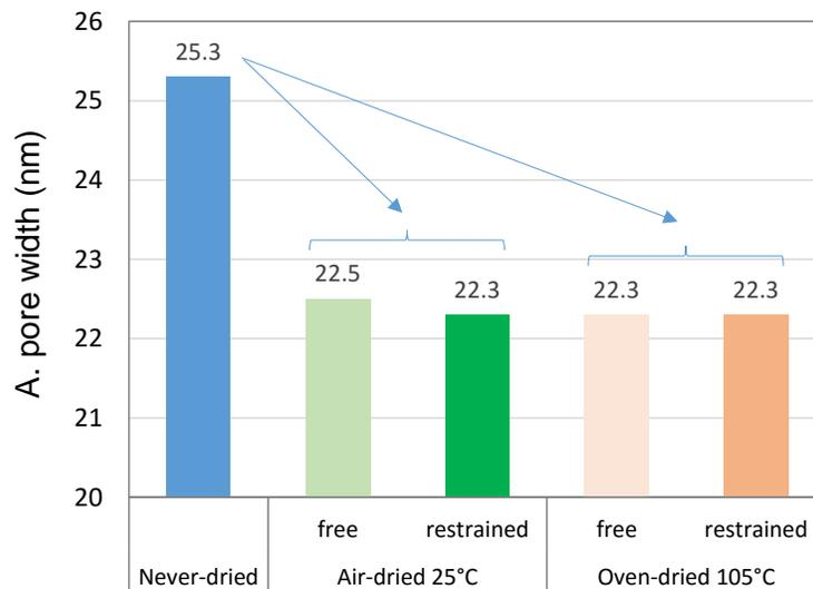
Fig. 15. Average pore size as measured by <sup>1</sup>H-NMR for never-dried, air-dried, and oven-dried pulps
