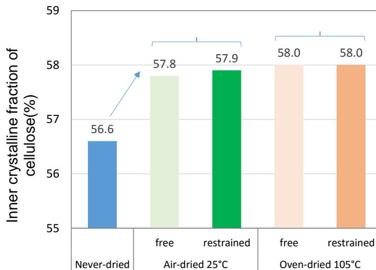
**Fig. 16.** Crystallinity of cellulose *via*  $^{13}\text{CP}$  MAS-NMR for never-dried, air-dried, and oven-dried pulps
