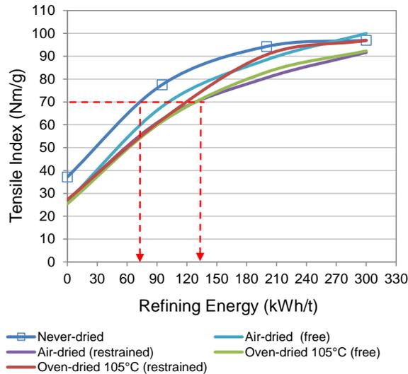
**Fig. 1.** Tensile index vs. specific refining energy for pulps refined in Voith Sulzer
