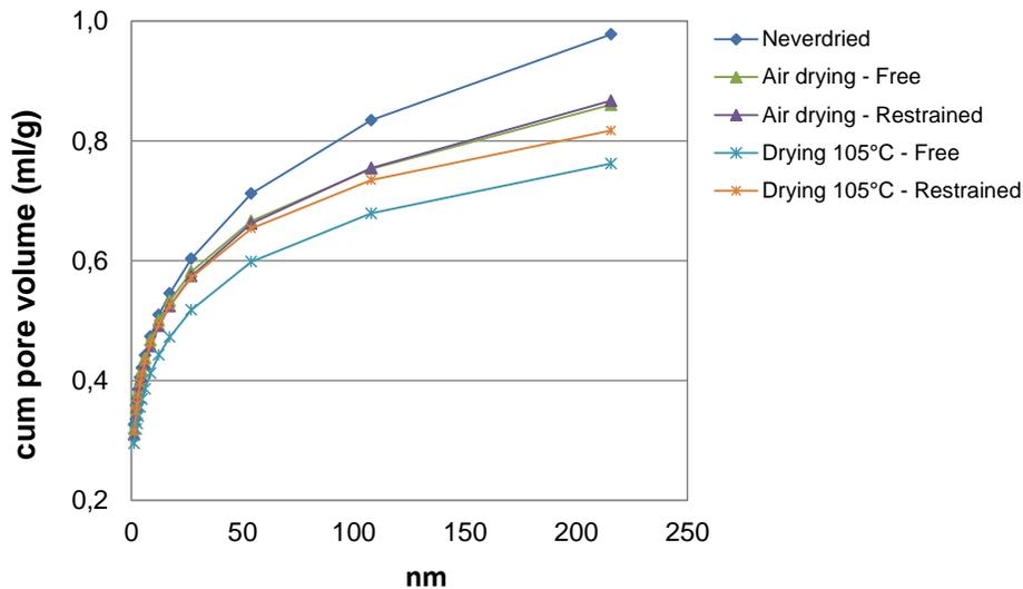
Fig. 14. Pore size distribution for never-dried, air-dried, and oven-dried pulps
