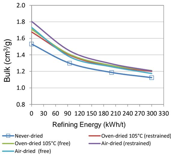
**Fig. 9.** Bulk vs. refining energy for pulps refined in Voith Sulzer
