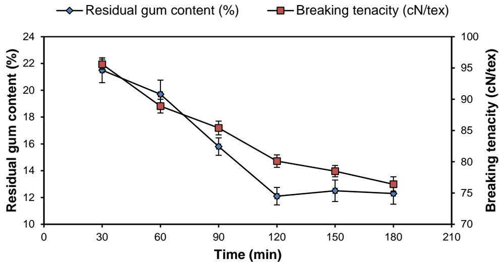
Fig. 3. Effect of react time for residual gum content and breaking tenacity
