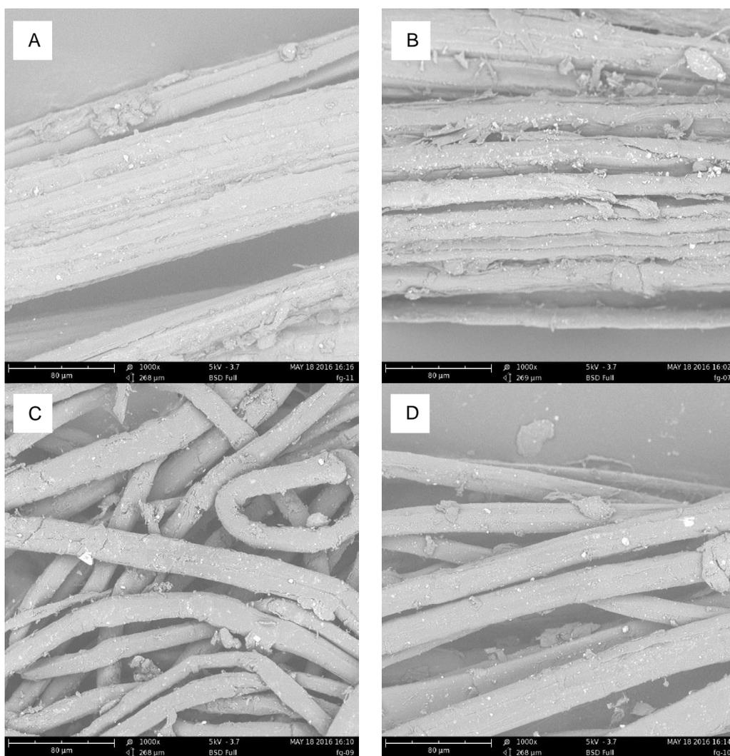
**Fig. 5.** Scanning electron micrograph of longitudinal view of (A) crude hemp (1000x), (B) enzymatic hydrolysis (1000x), (C) enzyme followed by alkali treated (1000x), and (D) bleached hemp fibers (1000x). Scale bars = 80  $\mu$ m in each micrograph
