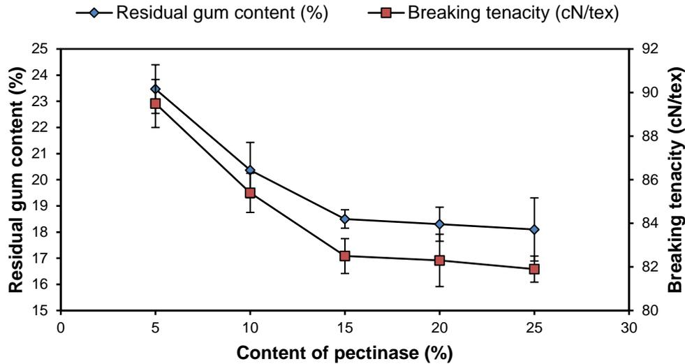
**Fig. 1.** Effect of pectinase content for residual gum content and breaking tenacity
