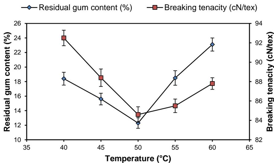
**Fig. 2.** Effect of temperature for residual gum content and breaking tenacity
