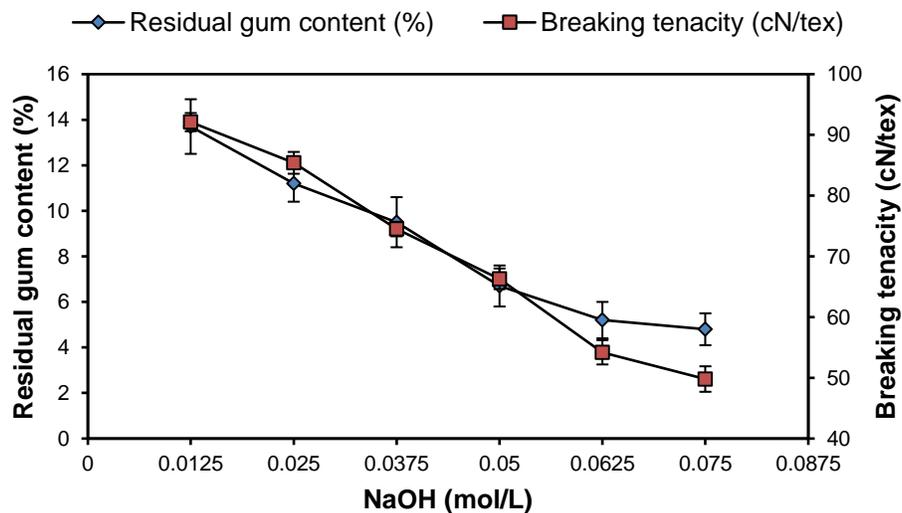
Fig. 4. Effect of NaOH content for residual gum content and breaking tenacity
