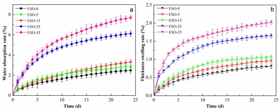
**Fig. 5.** The water absorption and thickness swelling rates of WPCs samples without and with various amounts of ESO
