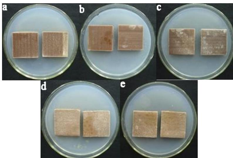
**Fig. 2.** The mould colonization of the WPCs with (a) 0 phr, (b) 5 phr, (c) 15 phr, (d) 25 phr, and (e) 35 phr ESO
