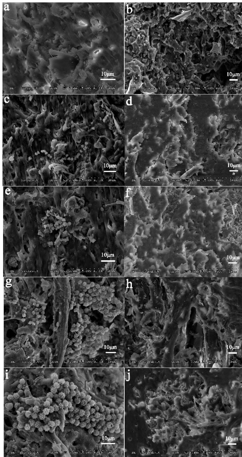
**Fig. 3.** The surface and fracture micro-morphology of algal growth of WPCs with (a) and (b) 0 phr ESO, (c) and (d) 5 phr ESO, (e) and (f) 15 phr ESO, (g) and (h) 25 phr ESO, and (i) and (j) 35 phr ESO. For each group, surface morphology is on the left, and fracture morphology is on the right
