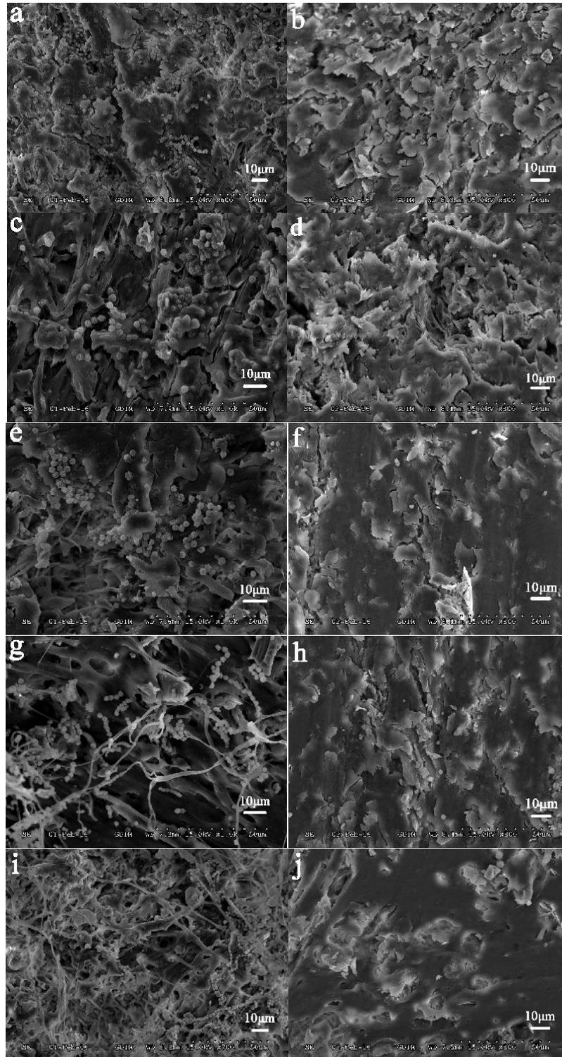
**Fig. 4.** The surface and fracture micro-morphology of mould growth for the WPCs with (a) and (b) 0 phr ESO, (c) and (d) 5 phr ESO, (e) and (f) 15 phr ESO, (g) and (h) 25 phr ESO, and (i) and (j) 35 phr ESO. For each group, surface morphology is on the left, and fracture morphology is on the right
