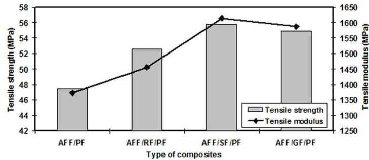
Fig. 3. Variation of the tensile properties of composites
