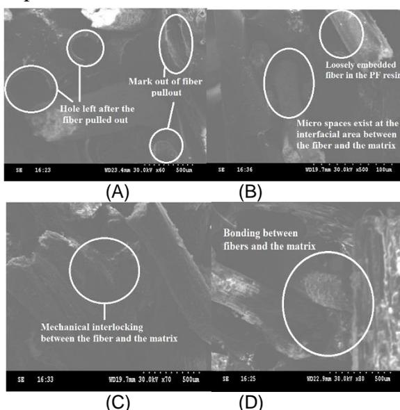
**Fig. 6.** SEM micrograph of a fractured surface of (A) the AFF/PF composite, (B) the AFF/RF/PF hybrid composite, and (C and D) the AFF/SF/PF hybrid composite after the tensile test
