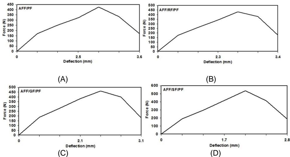
Fig. 4. Force and deflection curves of the flexural property of composites
