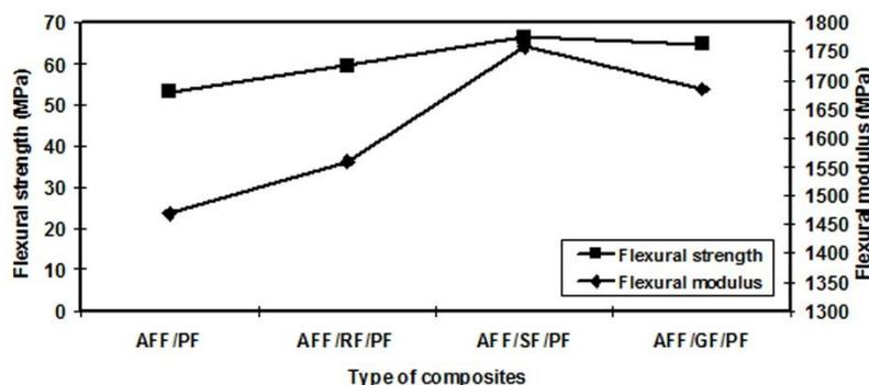
Fig. 5. Variation of the flexural properties of composites
