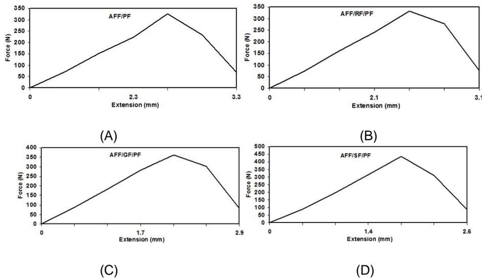
Fig. 2. Force and extension curves of tensile property of composites
