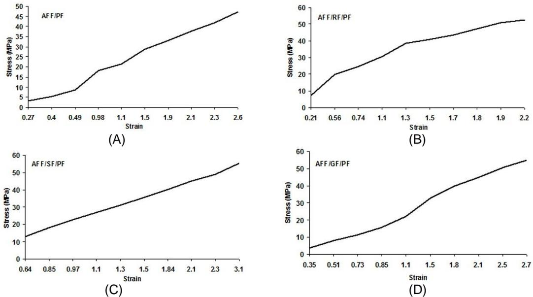
Fig. 1. Stress and strain curves of tensile property of composites
