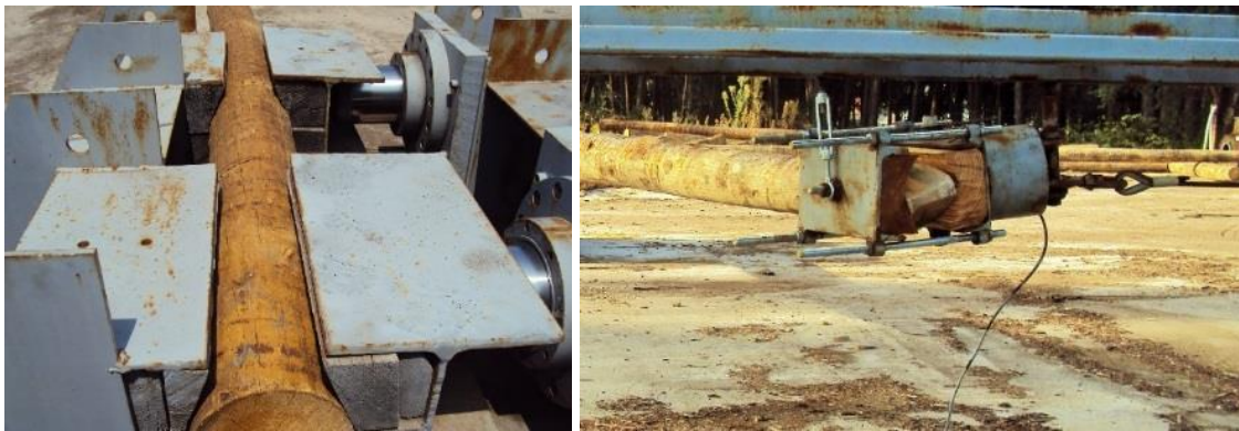
Fig. 2. Set up for cantilever tests: (left) wood clamps used at the bottom and (right) application of load at the tip
