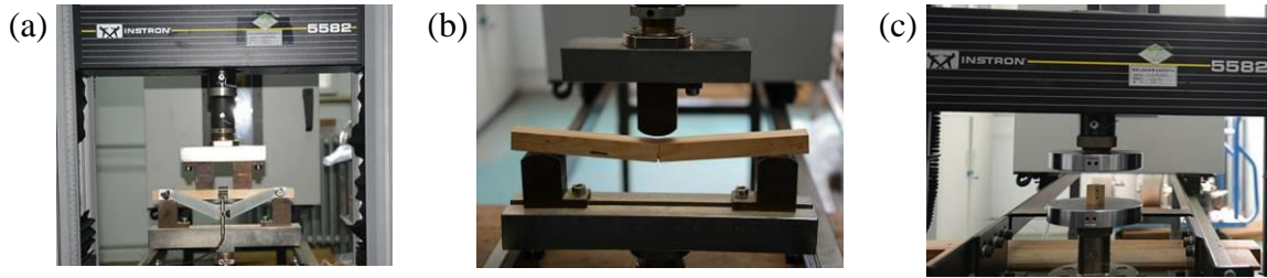
Fig. 3. Static mechanical tests: (a) MOE; (b) MOR; (c) UCS
