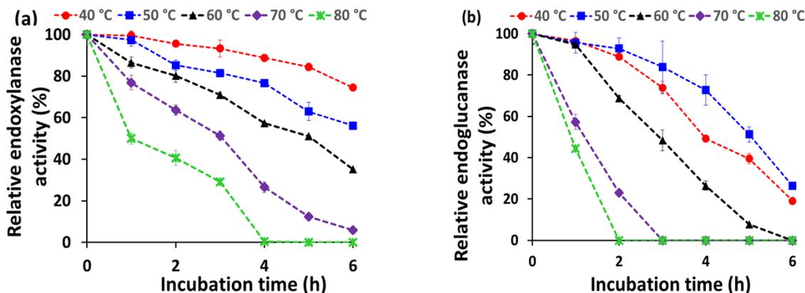
**Fig. 11.** The thermostability profiles of (a) endoxylanase and (b) endoglucanase. The enzymes were incubated at 40 °C (●), 50 °C (■), 60 °C (▲), 70 °C (◆), and 80 °C (x) for 6 h, and residual activities were detected at 1 h intervals. Data are presented as means of three replicates with SE.
