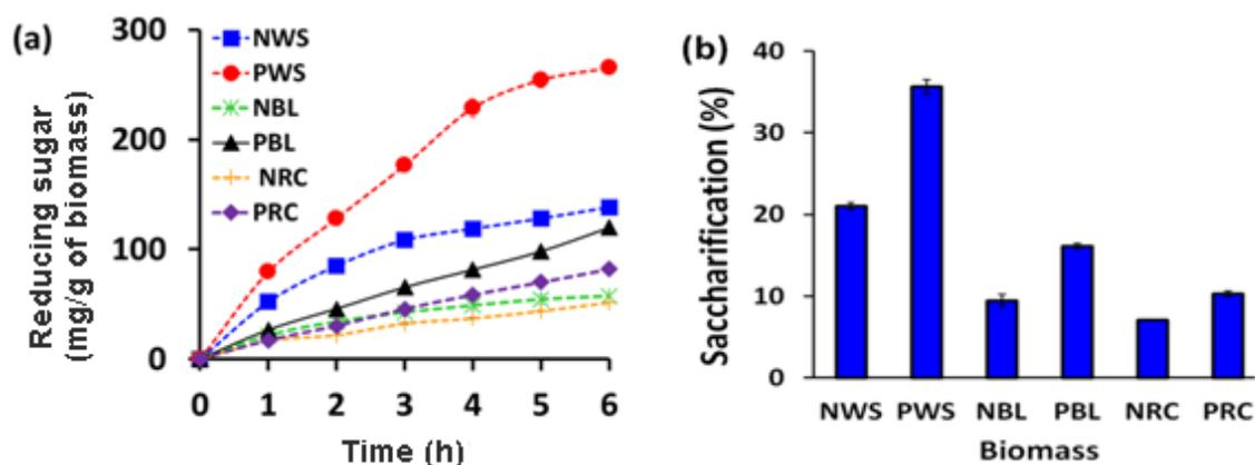
**Fig. 12.** (a) The reducing sugar and (b) saccharification rates, after hydrolysis of natural wheat straw (NWS), pretreated wheat straw (PWS), natural banana leaves (NBL), pretreated banana leaves (PBL), natural *R. communis* stalk (NRC), and pretreated *R. communis* stalk (PRC). Hydrolysis was performed at 60 °C for 6 h. Data are presented as means of three replicates with SE.
