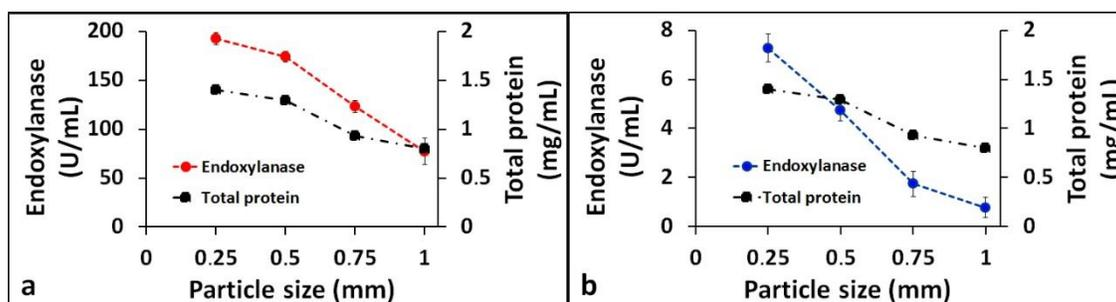
**Fig. 2.** Effect of the particle size of wheat straw on endoxylanase (a) and endoglucanase (b) production. Incubation was carried out in MS-YEM supplemented with wheat straw of different particle sizes as the primary carbon source at 30 °C and 150 rpm for 3 days. Data are presented as means of three replicates with SE.
