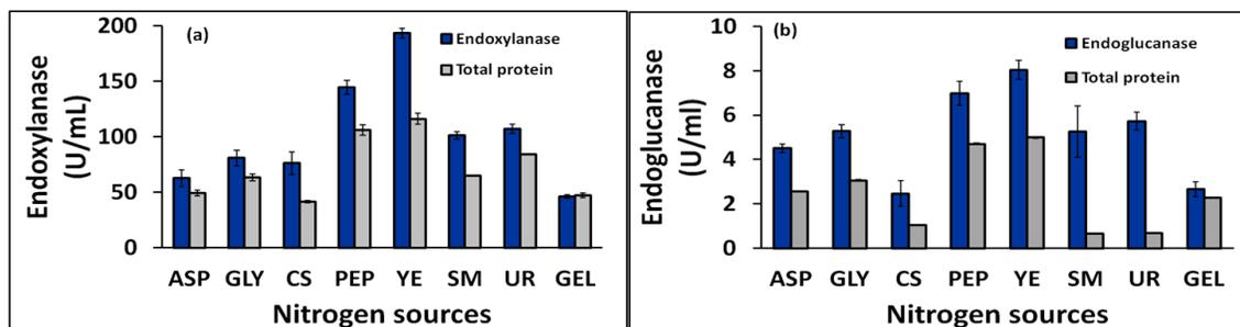
**Fig. 3.** The effect of different nitrogen sources on (a) endoxylanase and (b) endoglucanase production; incubation was carried out in MS-YEM supplemented with wheat straw ( $\leq 0.25$  mm) as the primary carbon source and with different nitrogen sources (Asparagine: ASP; Glycine: GLY; Casein: CS; Peptone: PEP; Yeast extract: YE; Soybean meal: SM; Urea: UR; Gelatine: GEL) at 30 °C and 150 rpm for 3 days; data are presented as means of three replicates with SEs
