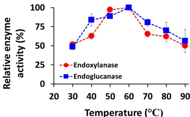
**Fig. 9.** Effect of the reaction temperature on endoxylanase and endoglucanase activity. After substrates (CMC and birchwood xylan) and enzymes incubated at specified temperatures for 10 min at pH 7.0, the DNS method was used to measure enzyme activity. Data are presented as means of three replicates with SE.
