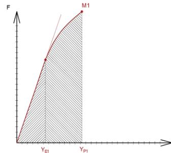
**Fig. 2.** Deflection at the proportional limit and at the point of rupture of wood species M1 with small plastic deformation
