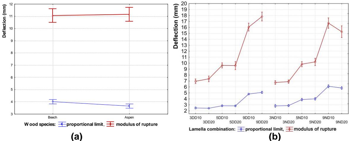
**Fig. 5.** The effect of the (a) wood species and (b) lamella combination on deflection at the proportional limit and at the point of rupture
