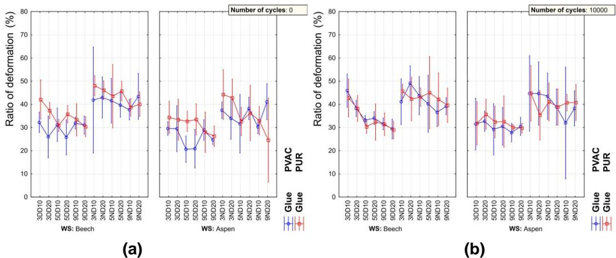
**Fig. 11.** Synergistic effect of the studied factors on the ratio of deflection (a – Number of cycles 0, b – Number of cycles 10,000)
