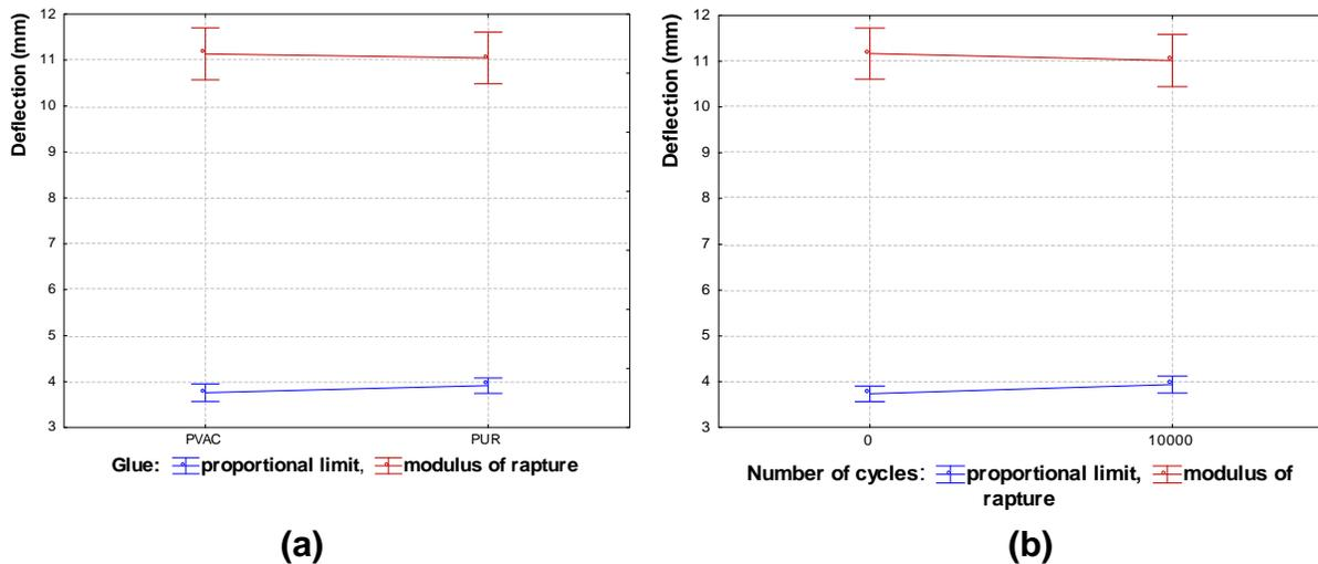
Fig. 6. The effect of the (a) glue and (b) number of cycles on deflection at the proportionality limit and at the point of rupture
