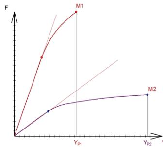
**Fig. 3.** The effect of the wood species on deflection at the point of rupture
