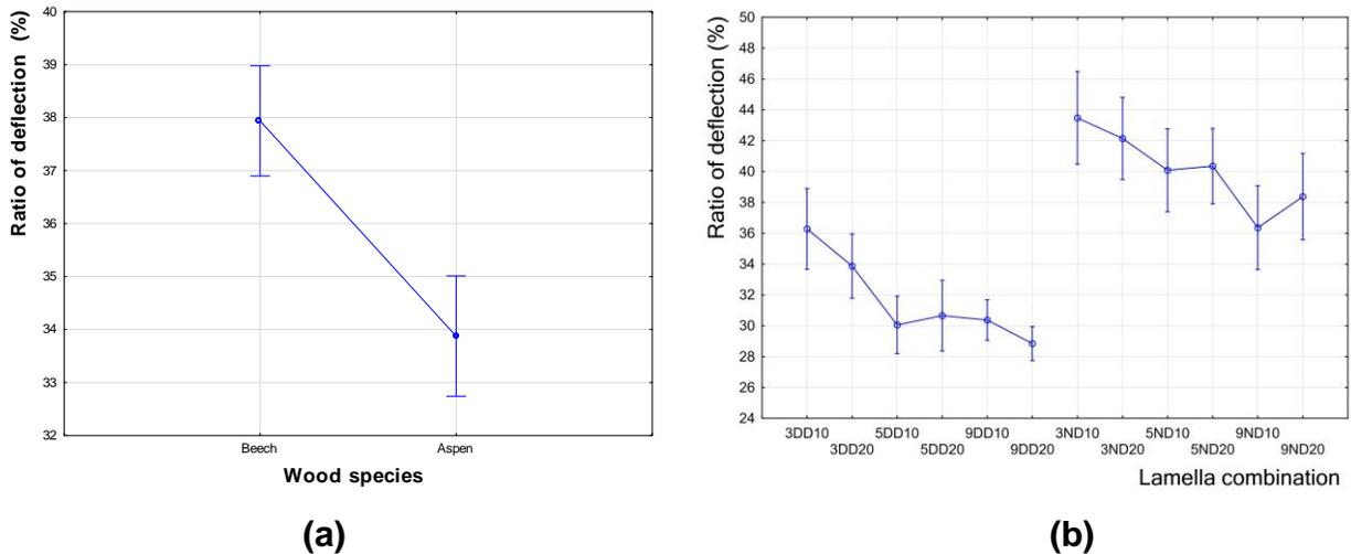
Fig. 9. The effect of the (a) wood species and (b) lamella combination on the ratio of deflection
