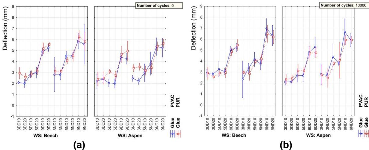
Fig. 7. Synergistic effect of the studied factors on the deflection at the proportionality limit (a – Number of cycles 0, b – Number of cycles 10000)
