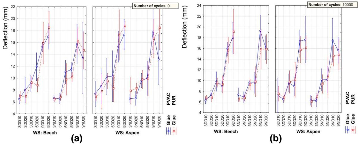
**Fig. 8.** Synergistic effect of the studied factors on the deflection at the point of rupture (a – Number of cycles 0, b – Number of cycles 10000)
