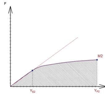
**Fig. 4.** Deflection at the proportional limit and at the point of rupture of wood species M2 with large plastic deformation
