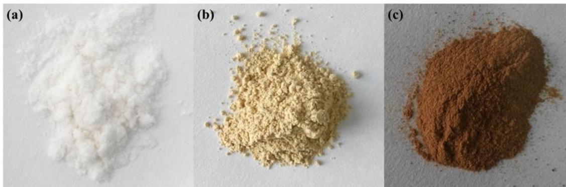
Fig. 3. The optical photographs of (a) cellulose, (b) hemicellulose, and (c) lignin prepared from P. sinese by microwave-assisted \text{H}_2\text{O}_2 -NaOH extraction. Reaction conditions: solid-liquid ratio of 1:25, 0.5% \text{H}_2\text{O}_2 , 4% NaOH, 75\text{ }^\circ\text{C} , and 4 h.
