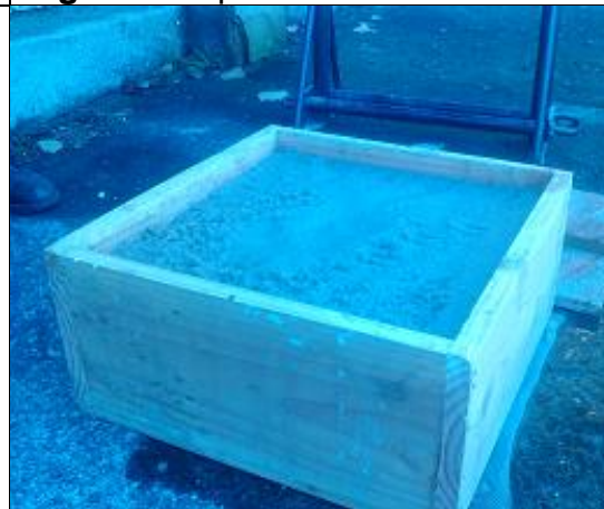
Fig. A4. Pre-pressing of disaggregated fibers
