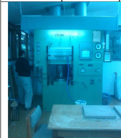
Fig. A5. Thermal pressing in hydraulic press
