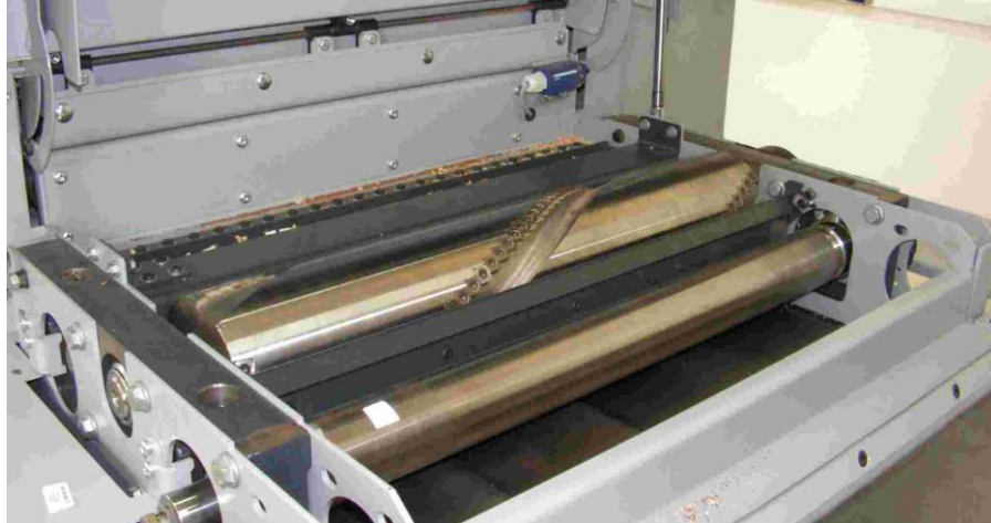
Fig. 1. (a) FELDER D963 thickening machine equipped with (b) a “silent power” cylindrical cutter head with helical cutters
