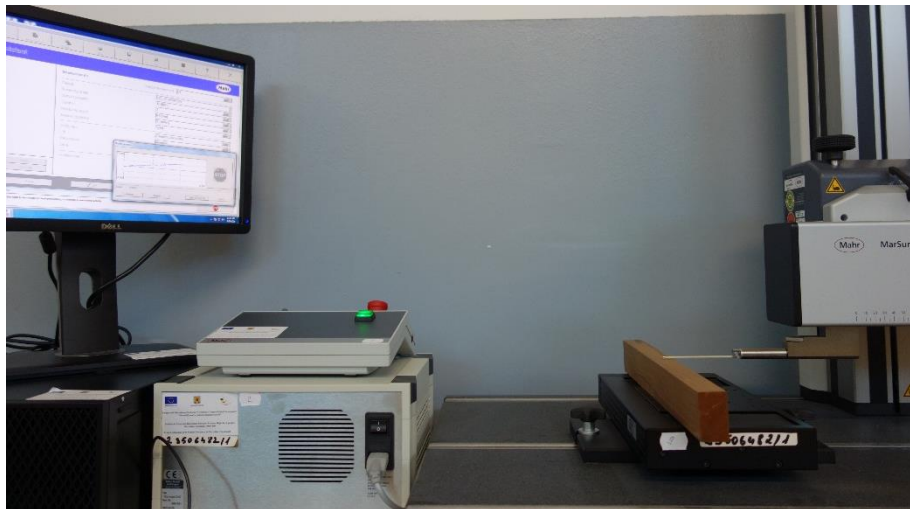
Fig. 2. Measuring the processing roughness by a MarSurf XT20 stylus
