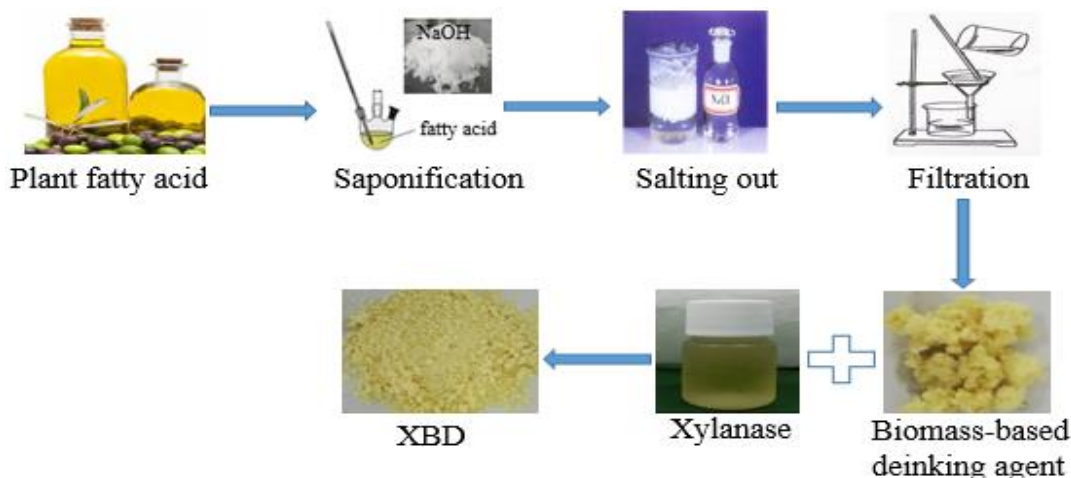
Fig. 1. The preparation process of XBD
