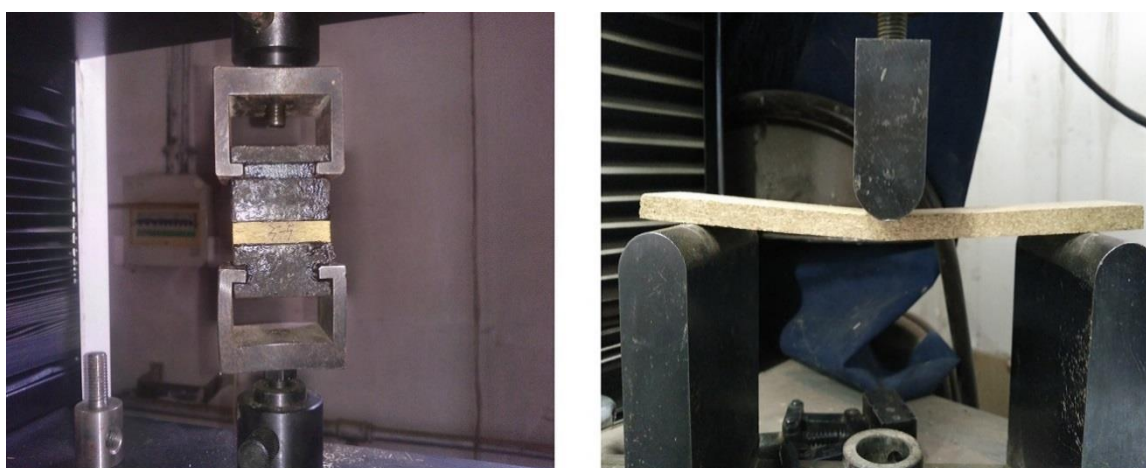
Fig. 1. Test of internal bond strength (L) and static bending properties (R)
