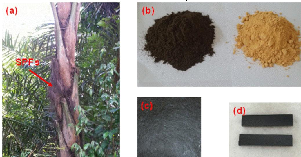
**Fig. 1.** (a) Sugar palm tree; (b) SPF and PF powders; (c) SPF/PF composite; (d) DMA samples
