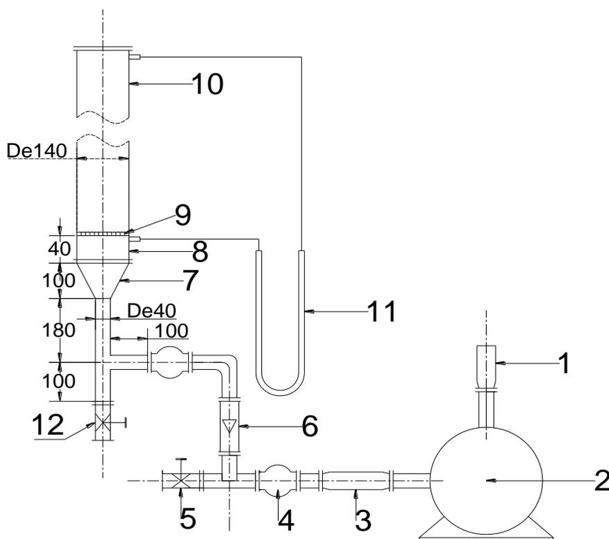
**Fig. 1.** Schematic diagram of a cold visualized fluidized bed experimental setup: 1-Import silencer; 2-Roots blower; 3- Export silencer; 4-Flexible joint; 5- Ball valve 1; 6-Rotameter; 7- Conic diffuse; 8- Plenum; 9- Gas distribution plate; 10- Riser; 11- U-Tube manometer; 12- Ball valve 2
