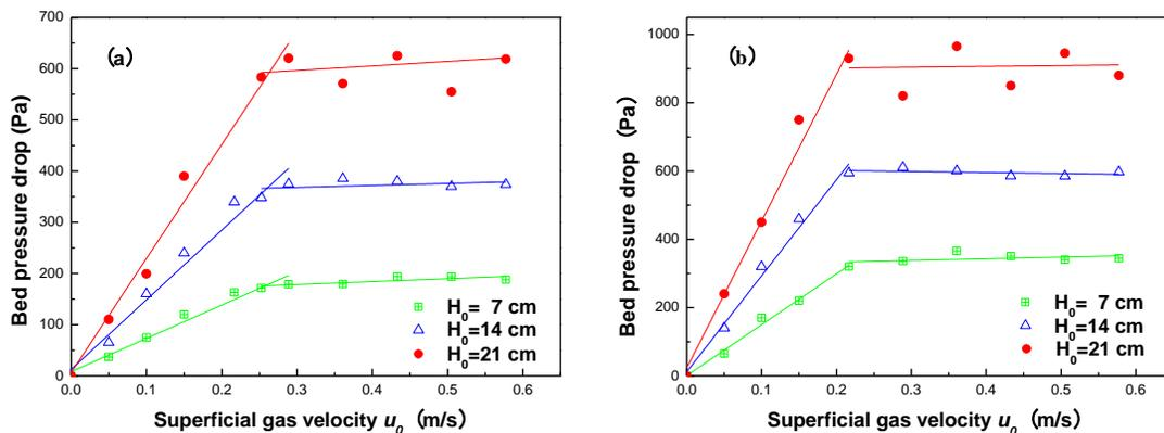
**Fig. 3.** Fluidization characteristic curves of biomass at various initial bed heights (a: rice husk,  $M = 3.7\%$ ; b: walnut shell,  $M = 3.3\%$ )
