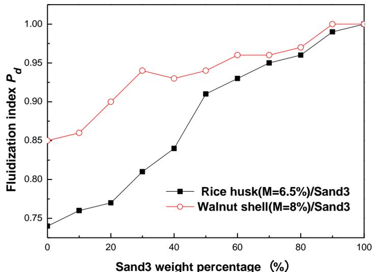
Fig. 9. Fluidization indices for mixed materials with different weight ratios
