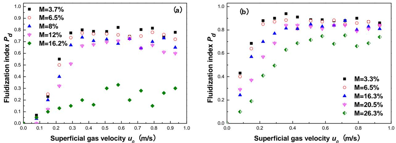
Fig. 4. Fluidization characteristic curves for biomass with various moisture contents (a: rice husk; b: walnut shell)
