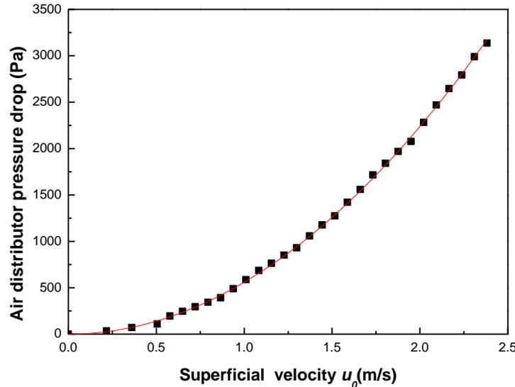
**Fig. 2.** Curve of resistance characteristics of gas distributor
