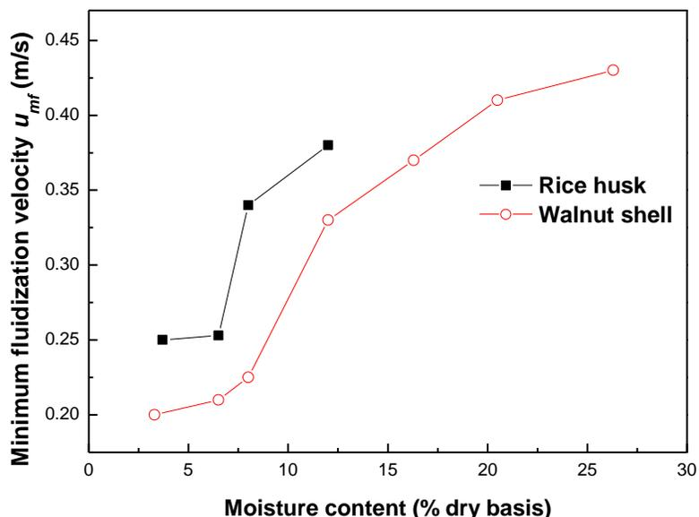
Fig. 5. The minimum fluidization velocity of biomass with various moisture contents
