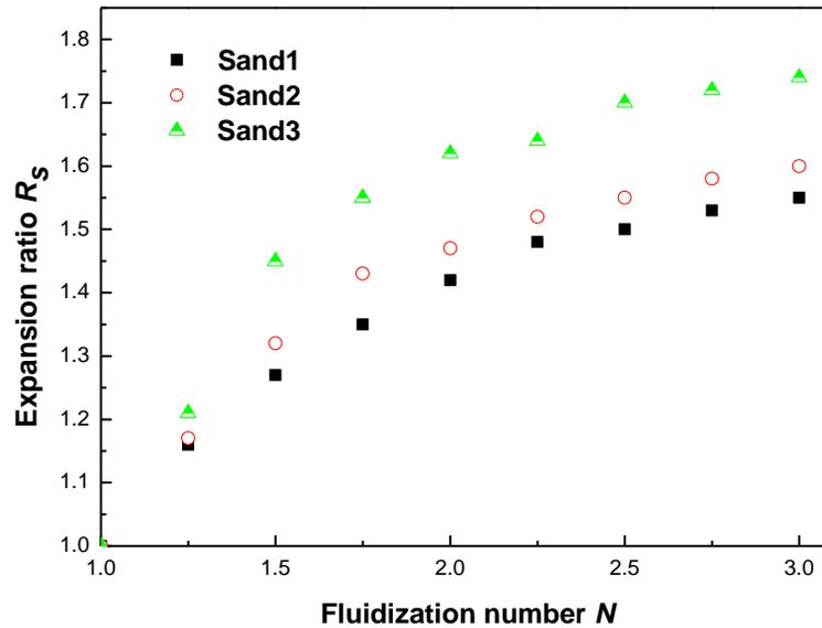
Fig. 7. Bed expansion ratio for different fluidization numbers
