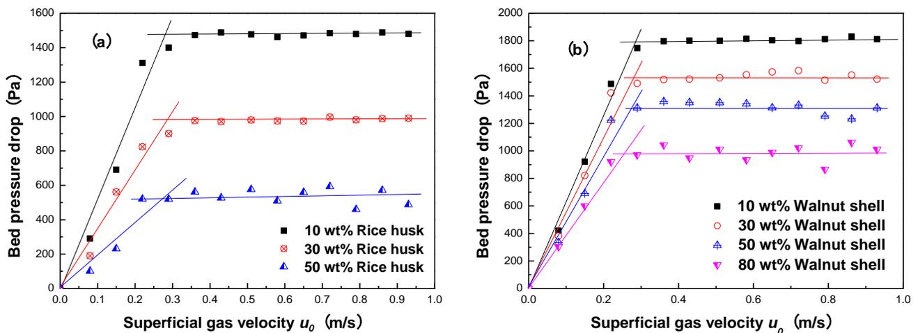
Fig. 8. Mixed fluidization characteristic curve of biomass/sand-3 (a: rice husk,  $M = 6.5\%$ ; b: walnut shell,  $M = 8\%$ )
