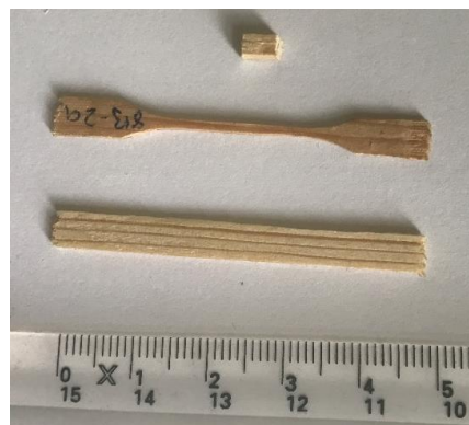
Fig. 2. The bending, tensile, and compression test samples. Numbers on the ruler correspond to cm units, and the fine scale markings correspond to mm units.
