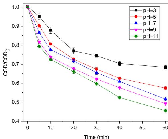
**Fig. 3.** Effect of initial pH on ozonation efficiency
