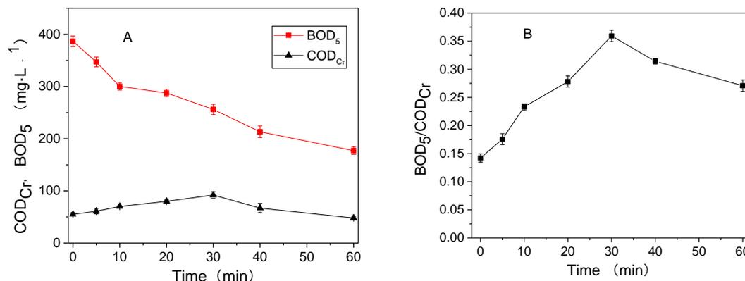
Fig. 7. Variation of COD<sub>Cr</sub>, BOD<sub>5</sub>, and BOD/COD ratio of BTPW during ozonation
