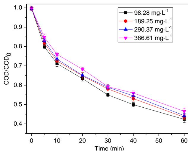
Fig. 4. Effect of initial  $\text{COD}_{\text{Cr}}$  concentration on ozonation efficiency
