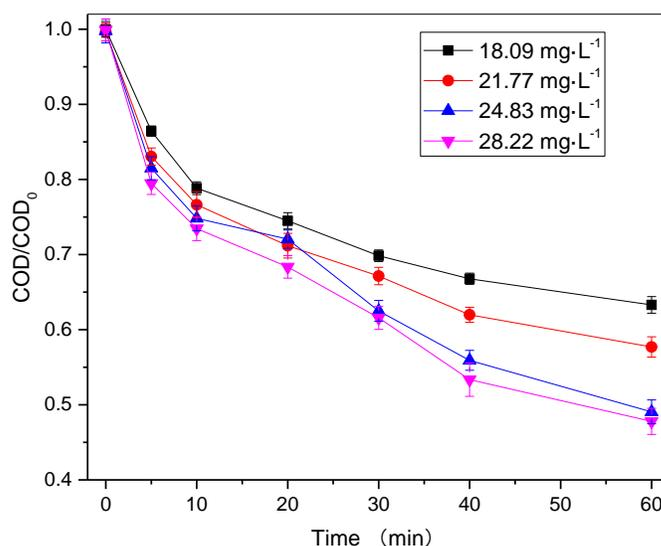
Fig. 6. Effect of ozone concentration on ozonation efficiency
