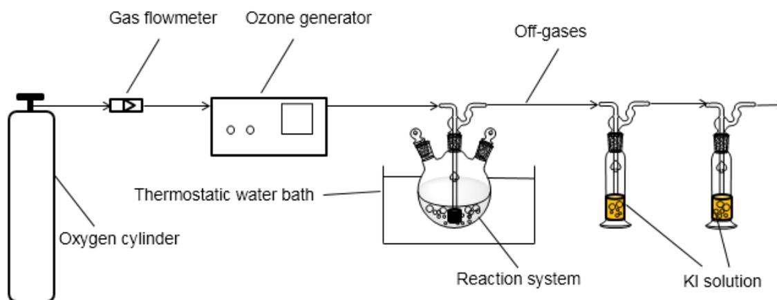
Fig. 1. Scheme of ozonation setup
