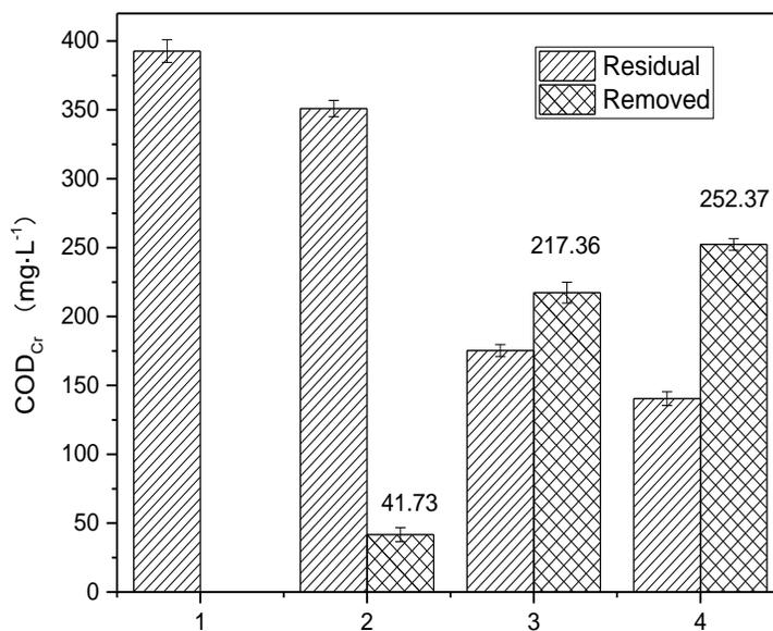
**Fig. 9.** COD<sub>Cr</sub> elimination of the BTPW by biotreatment and combination of ozonation with biotreatment: 1: raw BTPW; 2: biotreatment alone; 3: integrated ozonation for 30 min with biotreatment; and 4: integrated ozonation for 60 min with biotreatment
