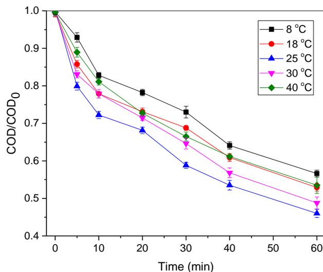
Fig. 5. Effect of temperature on ozonation efficiency
