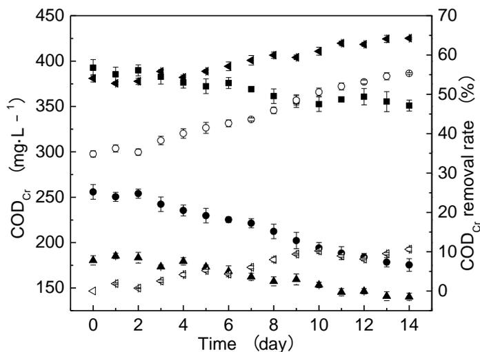
Fig. 8. Changes of COD<sub>Cr</sub> and COD<sub>Cr</sub> removal rates of the BTPW during biological treatment: (■) COD for non-ozonized BTPW, (●) COD for BTPW ozonized for 30 min, (▲) COD for BTPW ozonized for 60 min, (◁) COD removal rate for non-ozonized BTPW, (○) COD removal rate for BTPW ozonized for 30 min, and (◀) COD removal rate for BTPW ozonized for 60 min
