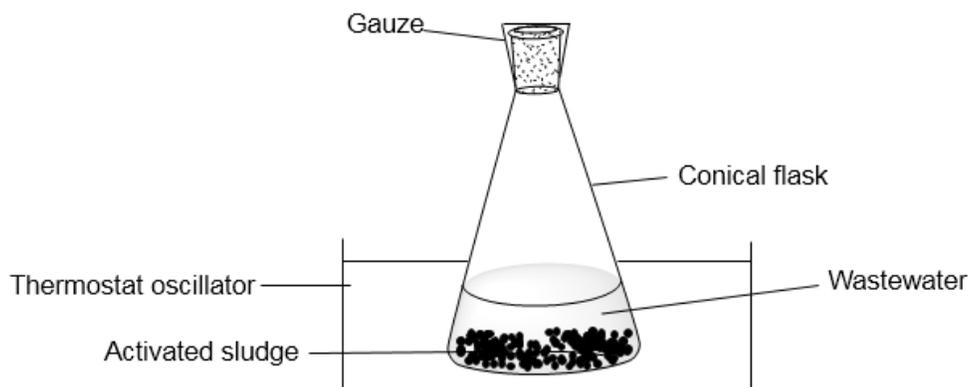
**Fig. 2.** Scheme for biological treatment setup
