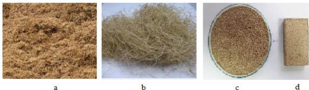
Fig. 1. OPEFB fibre: (a) Dirty fibres, (b) Washed fibres, (c) Crushed fibres, and (d) Compressed fibres
