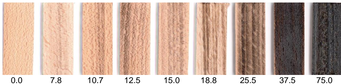
Fig. 2. Laser treated beech wood surfaces with different irradiation doses H ( \text{J}/\text{cm}^2 ).
