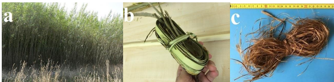
Fig. 1. (a) SRC with young willow trees, (b) fresh bark bundle, and (c) extracted fiber bundle
