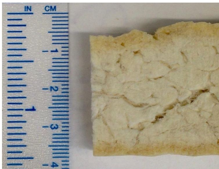
Fig. 1. Close-up optical photograph of sawn acrylic composite, with the exterior layers visible top and bottom
