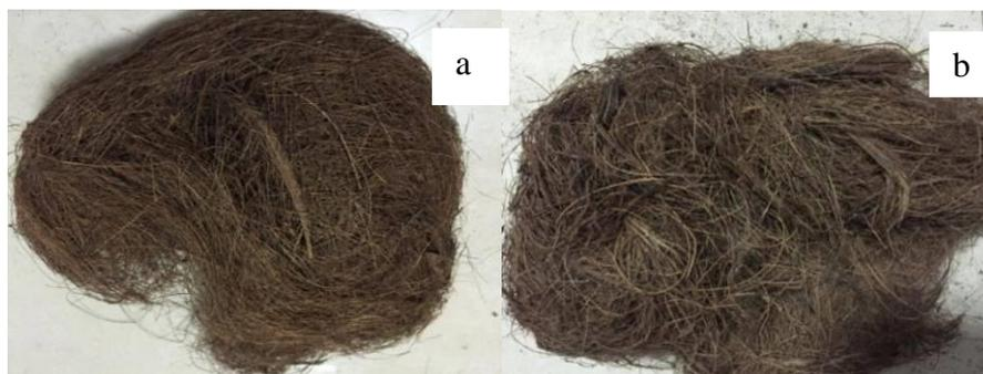
**Fig. 2.** (a) Palm leaf sheath fiber; (b) palm petioles fiber
