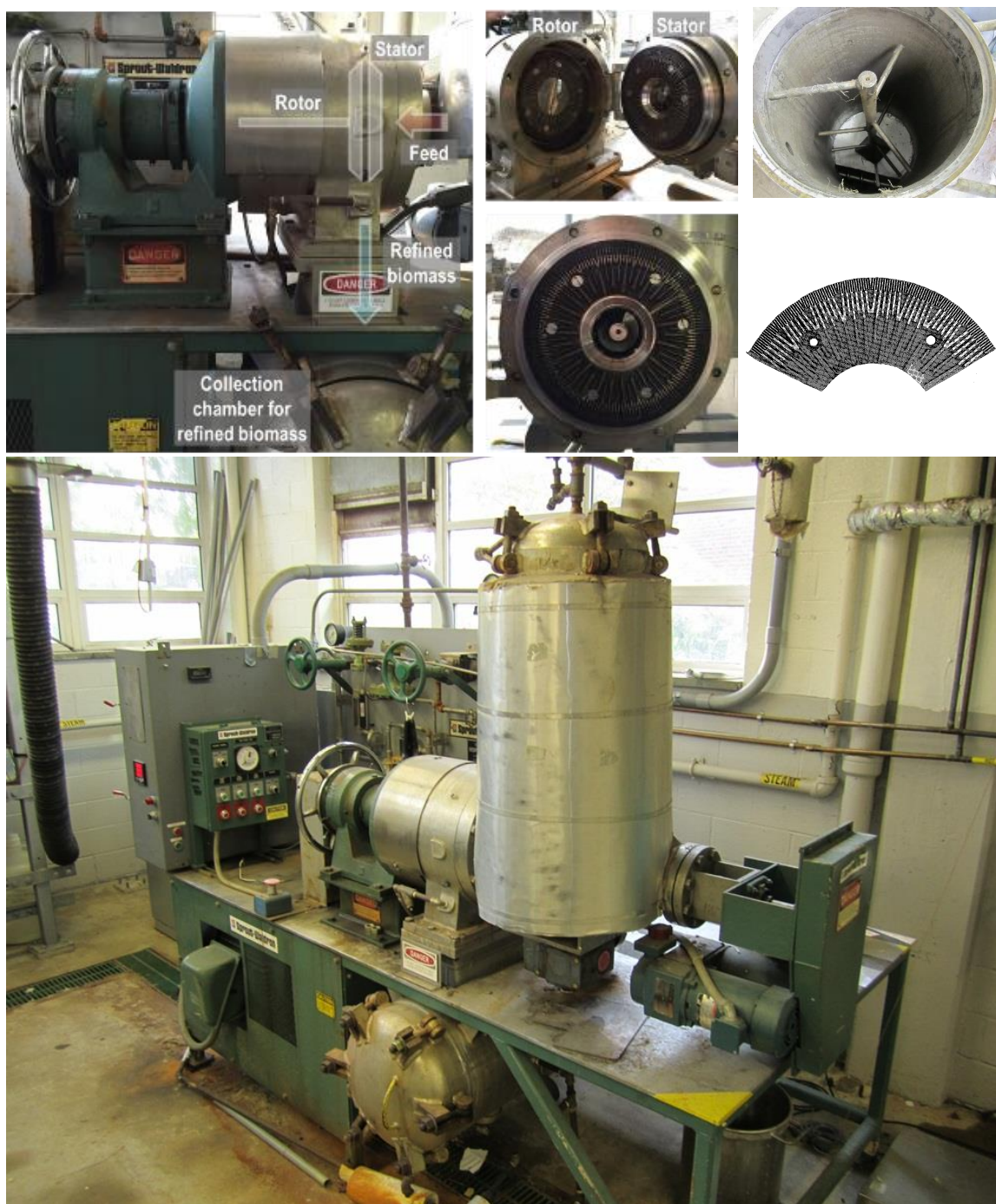
Fig. 2. NCSU pilot scale refining apparatus; the unrefined biomass was fed via the screw feeder into the refining zone, and the refined biomass was collected in the bottom vessel.
