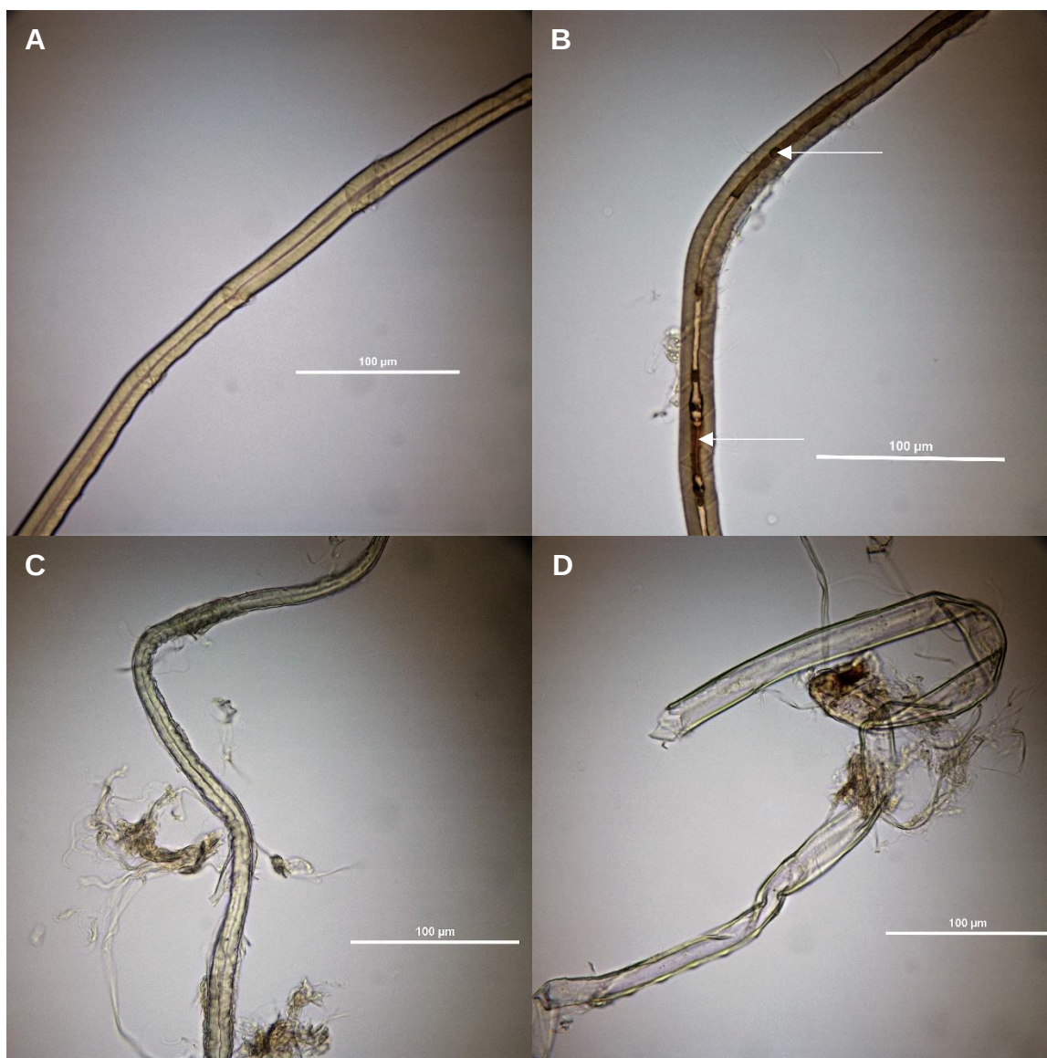
Fig. 4. Light microscope images of a) unrefined, and b) 5% cons, 0.05-mm gap, 150 °C, c) 20% cons, 0.03-mm gap, 30 °C, and d) 20% cons, 0.03-mm gap, 30 °C mechanically refined sodium carbonate pretreated biomass. The arrows in Fig. 4b reveal material deposits (presumably lignin) in the 150 °C sample that were not seen in any other condition. It is expected that this redistribution of lignin changed the enzyme accessibility and explained the reduction in 150 °C refined biomass digestibility compared with the other refined conditions.
