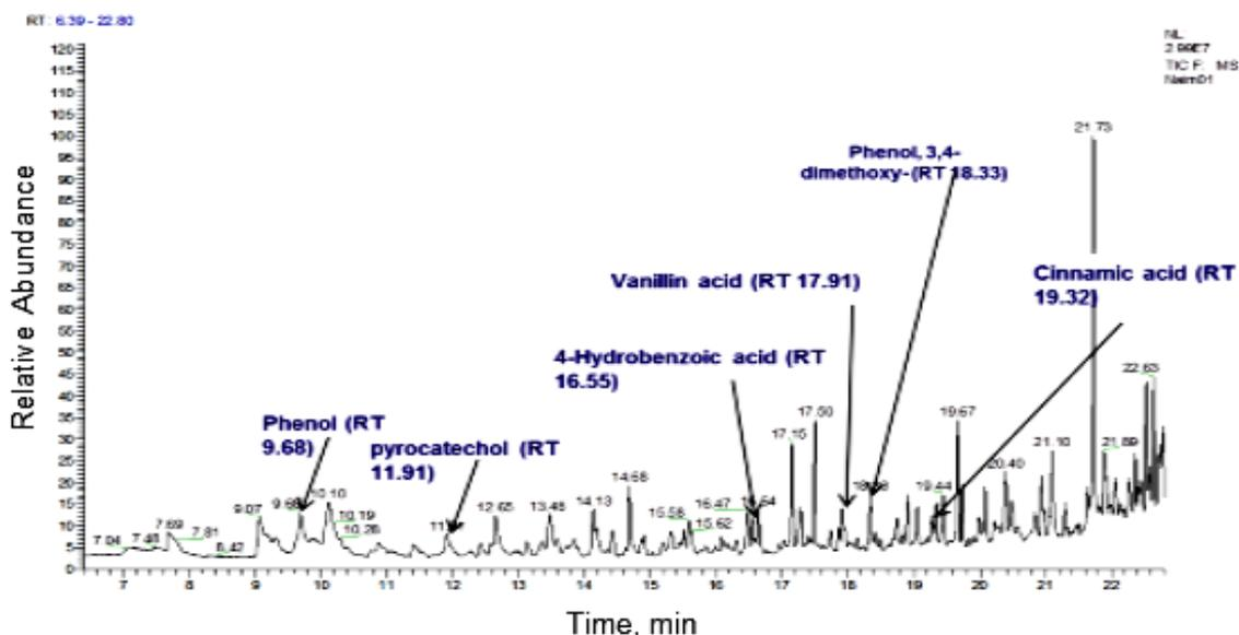
**Fig. 1.** GC-MS analyses for the determination of the phenolic acids in EFBs using iso-octane as the background solvent for the development of the calibration curve
