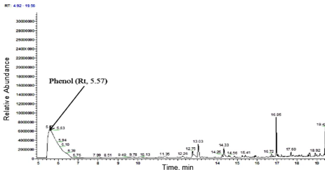
**Fig. 2.** GC-MS analyses for the determination of the phenolic acids in EFB using ethanol as the background solvent for the development of the calibration curve
