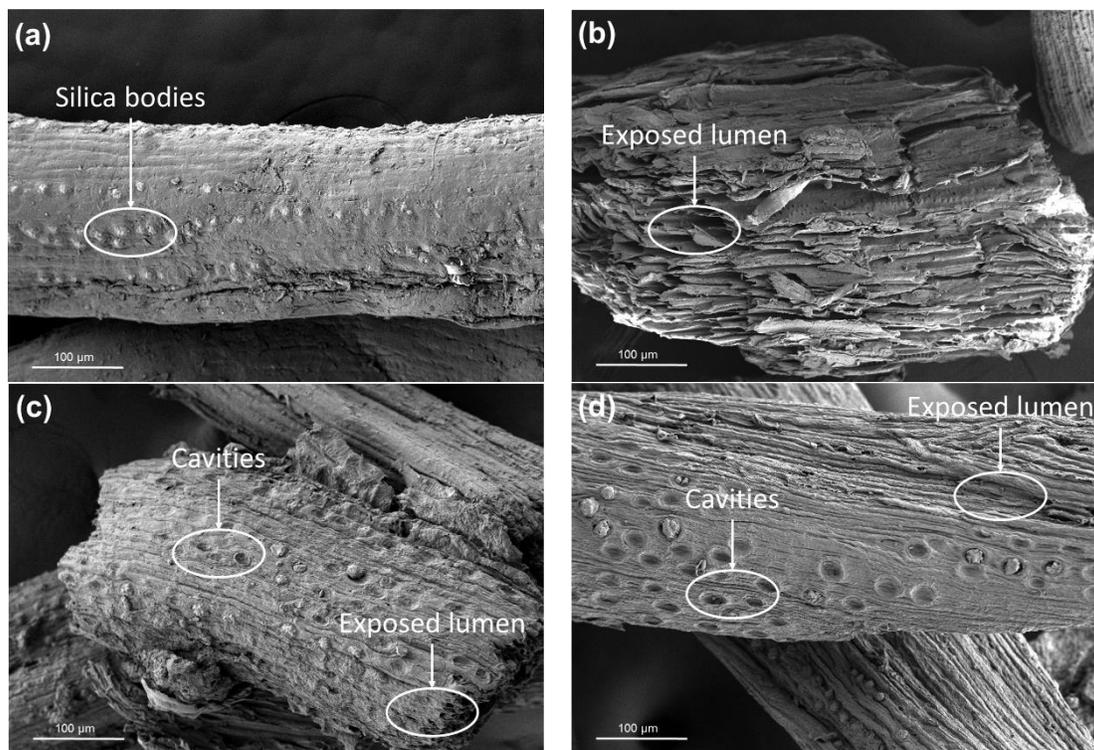
**Fig. 3.** Surface morphology of (a) raw and delignified EFB by Fenton reagents of (b) Fe(III), (c) Fe<sub>3</sub>O<sub>4</sub>, and (d) *in situ* reaction of Fe(0) (Fenton reagent: 8 mg/L; EFB fibers: 1 g; H<sub>2</sub>O<sub>2</sub>: 200 mmol)
