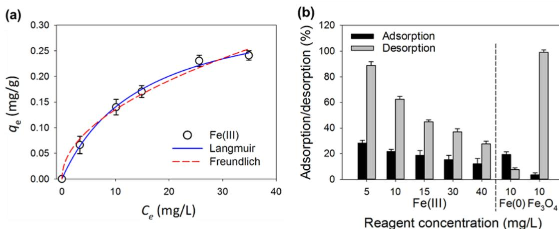
**Fig. 1.** The optimization of deposited Fenton reagents in (a) the uptake of Fe(III) ion adsorption isotherm of non-linear Langmuir and Freundlich and (b) adsorption/desorption behavior of Fenton reagent on EFB fibers (Fe(III): 5 mg/L to 40 mg/L; EFB fibers: 1 g)
