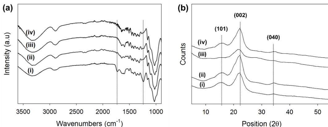
**Fig. 4.** Characterization of (i) raw and delignified EFB fibers in assisted Fenton reagents [(ii): Fe(III), (iii): Fe(0), (iv): Fe<sub>3</sub>O<sub>4</sub>] on (a) FTIR spectra and (b) XRD (Fenton reagent: 8 mg/L; EFB fibers: 1 g; H<sub>2</sub>O<sub>2</sub>: 200 mmol)
