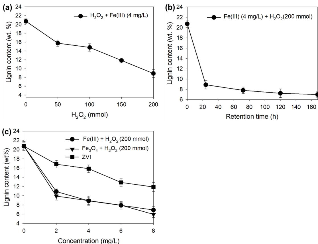
**Fig. 2.** The delignification of EFB fibers (a) in assisted of Fe(III) with different  $H_2O_2$  concentrations (Fe(III): 4 mg/L; EFB fibers: 1 g;  $H_2O_2$ : 50-200 mmol)., (b) oxidation retention time (Fe(III): 4 mg/L; EFB fibers: 1 g;  $H_2O_2$ : 200 mmol).and (c) with different Fenton reagents (Fenton reagents: 2-8 mg/L; EFB fibers: 1 g;  $H_2O_2$ : 200 mmol)
