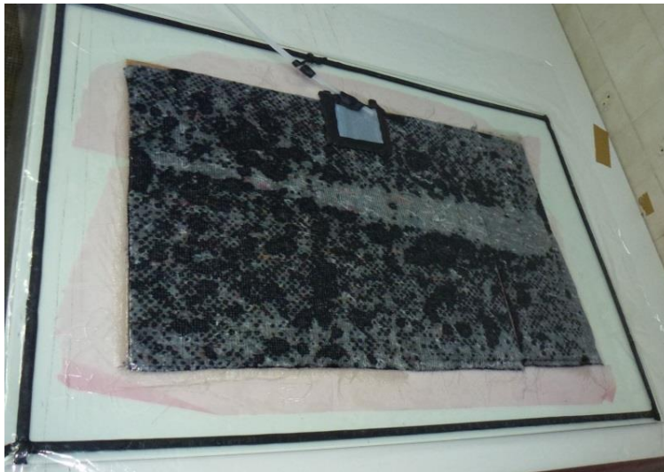
Fig. 1. Sandwich composite sheet manufactured using the vacuum bagging method
