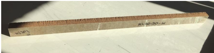
Fig. 4. Sample with Corecork NL20 core after four-point flexural test
