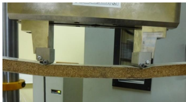
Fig. 8. Cracking of the cladding material (glass-epoxy laminate) in the sample with NL20 during the fatigue test
