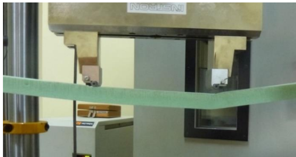
Fig. 7. Asymmetrical cracking of the cladding surface (glass-epoxy laminate) in the sample with Divinycell H60 during the fatigue test
