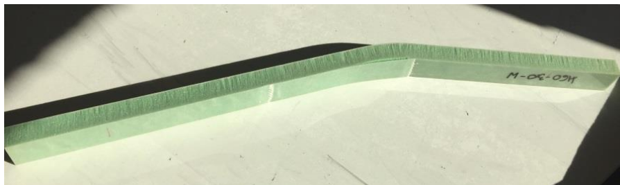
Fig. 5. Sample with synthetic Divinycell H60 foam core after four-point flexural test
