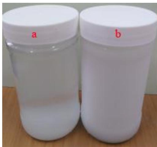
**Fig. 3.** Aqueous solutions of (a) bleached fibers (BF) and (b) cellulose nanofibers (NCF)
