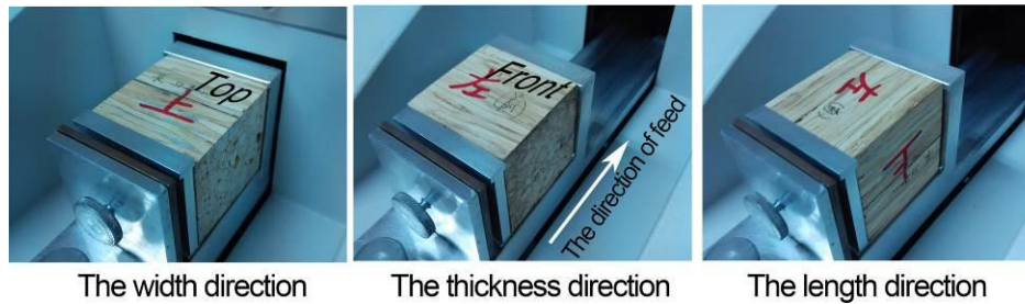
Fig. 4. The experimental process of density distribution
