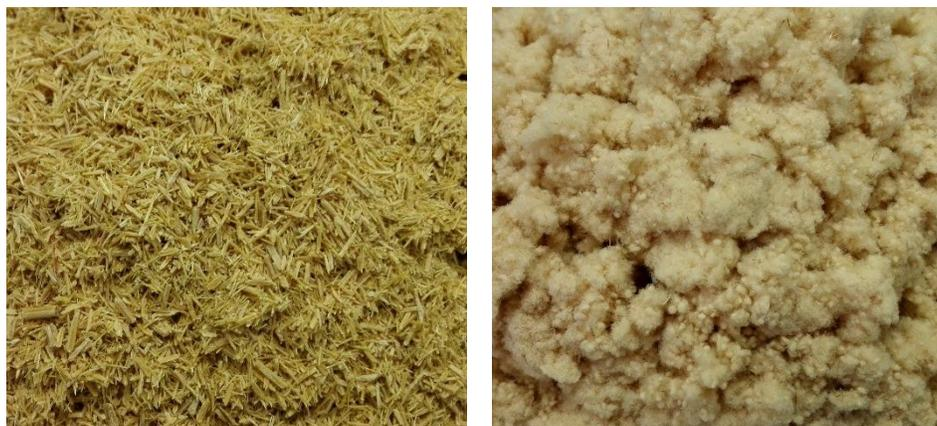
**Fig. 2.** Photographs of the bamboo residue (left) and pulp (right)
