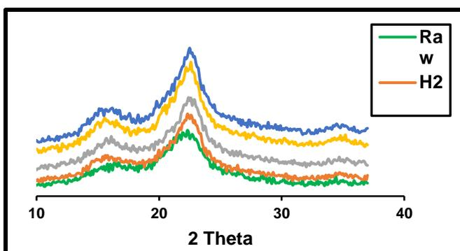
**Fig. 3.** XRD diagram of the raw RH and RH high-pressure steam pretreated at 160 °C (H2), 180 °C (H3), 200 °C (H4), and 220 °C (H5) for 7 min
