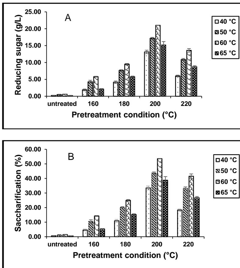
**Fig. 5.** Effect of temperature on the (A) reducing sugar production and (B) saccharification degree of high-pressure steam pretreated RH
