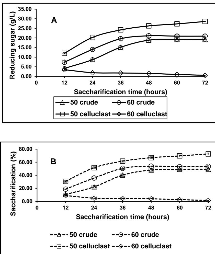
**Fig. 6.** Effect of time on the (A) reducing sugar production and (B) saccharification degree for hydrolysis conducted at 50 and 60 °C. RH pretreated at 200 °C for 7 min was used.
