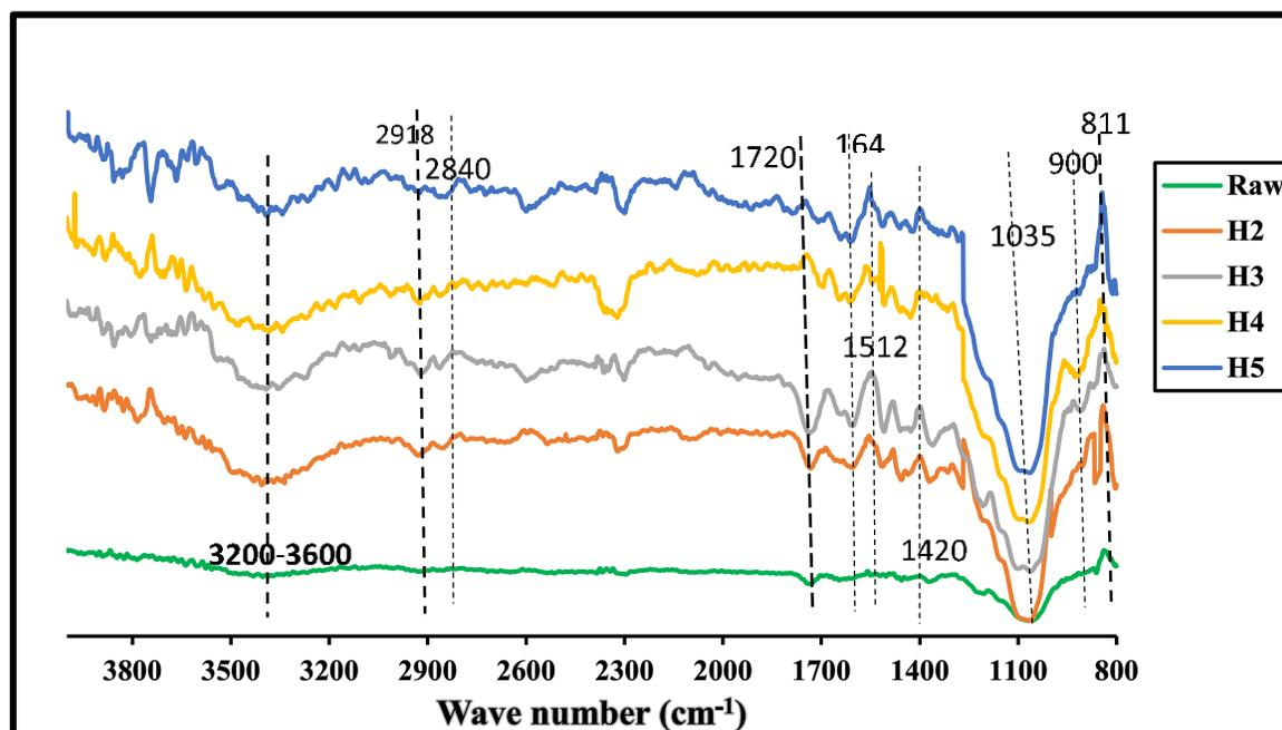
**Fig. 2.** FTIR spectra of the raw RH and RH high-pressure steam pretreated at  $160\text{ }^{\circ}\text{C}$  (H2),  $180\text{ }^{\circ}\text{C}$  (H3),  $200\text{ }^{\circ}\text{C}$  (H4), and  $220\text{ }^{\circ}\text{C}$  (H5) for 7 min
