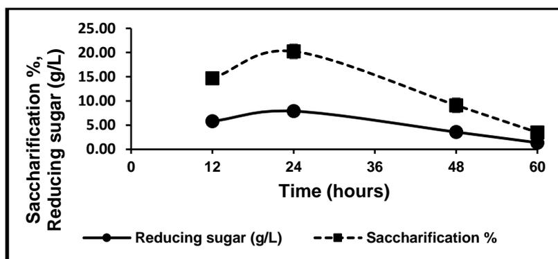
**Fig. 7.** Reducing sugar production and saccharification from the second-stage hydrolysis process. Hydrolysis was conducted at 60 °C on the RH pretreated at 200 °C for 7 min
