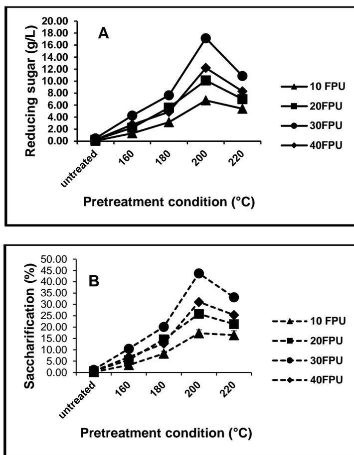
**Fig. 4.** Effect of enzyme loading on (A) reducing sugar production and (B) saccharification of high pressure steam pretreated rice husk
