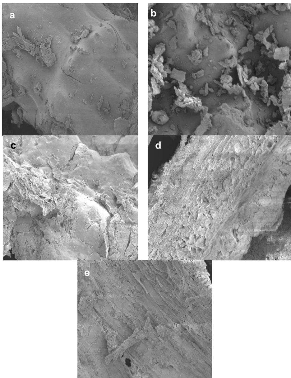
**Fig. 1.** SEM micrographs at 1000x magnification of the (A) untreated RH and RH samples pretreated at (B) 160 °C, (C) 180 °C, (D) 200 °C, and (E) 220 °C for 7 min.
