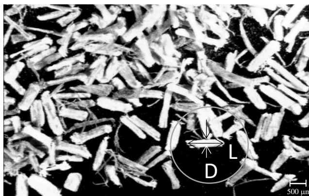
Fig. 1. Retained particles in 40-mesh sieve. Micrograph (10X lens)
