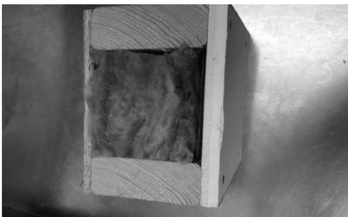
**Fig. 1.** Miniature model of a inside residential wall with the fiberglass batt insulation in between the 2x4 lumber
