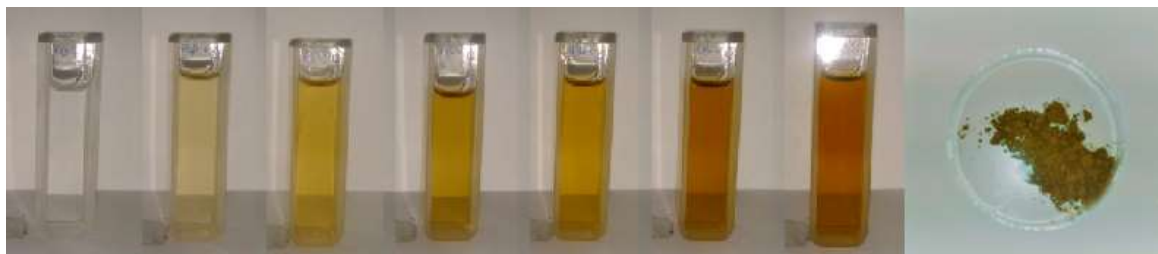
Fig. 1. Pure DES 1, solubilized lignin with different concentration of lignins, and straw lignin
