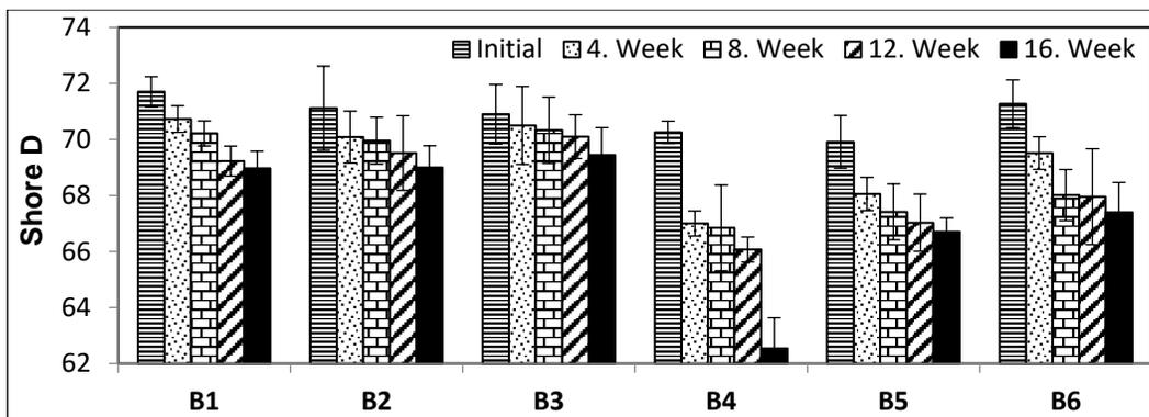
Fig. 7. Hardness of composite samples exposed to *T. versicolor*
