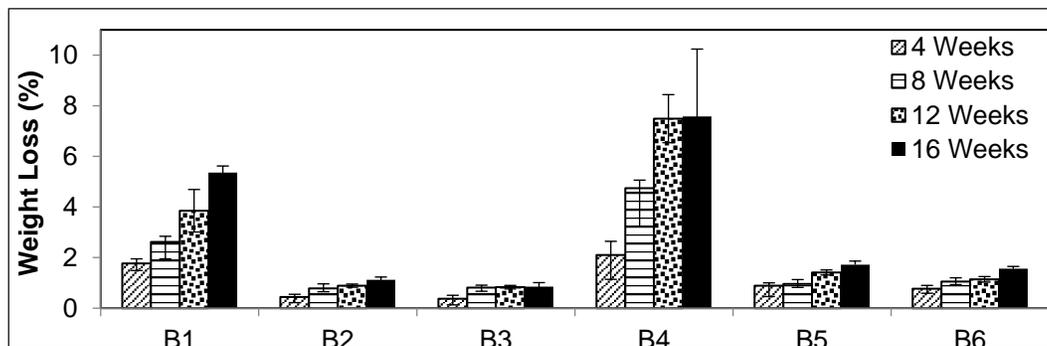
Fig. 1. Weight loss of composite samples exposed to *P. placenta*
