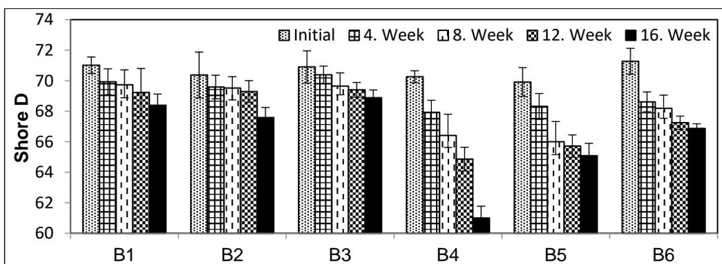
Fig. 5. Hardness of composite samples exposed to *P. placenta*
