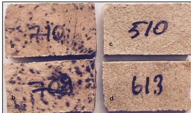
**Fig. 4.** Appearance of the composite samples exposed to *P. placenta* after 16 weeks of fungal decay: a,b) sample B4; c) sample B5; d) sample B6
