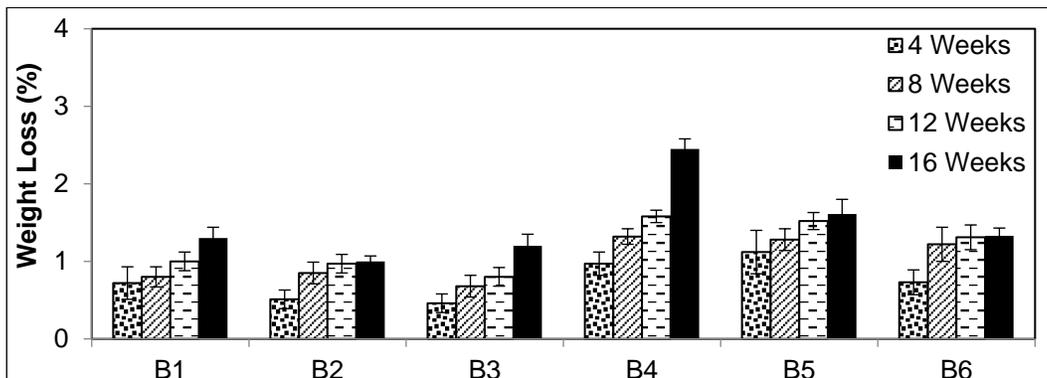
Fig. 3. Weight loss of composite samples exposed to *T. versicolor*
