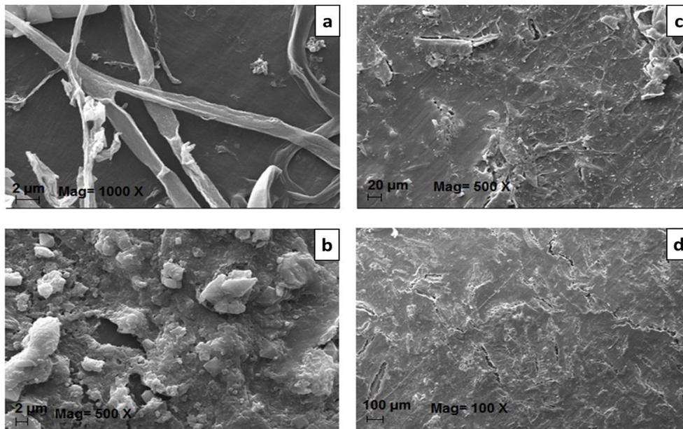
Fig. 8. SEM images of the composite samples after exposed to *P. placenta*: a) fungus mycelium; b) distribution of zinc borate; c, d) surface cracks.
