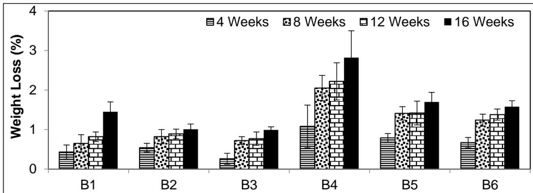
Fig. 2. Weight loss of composite samples exposed to *C. puteana*
