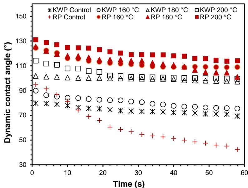
**Fig. 4.** Dynamic contact angle of Korean white pine (KWP) and royal paulownia (RP) before and after heat treatment
