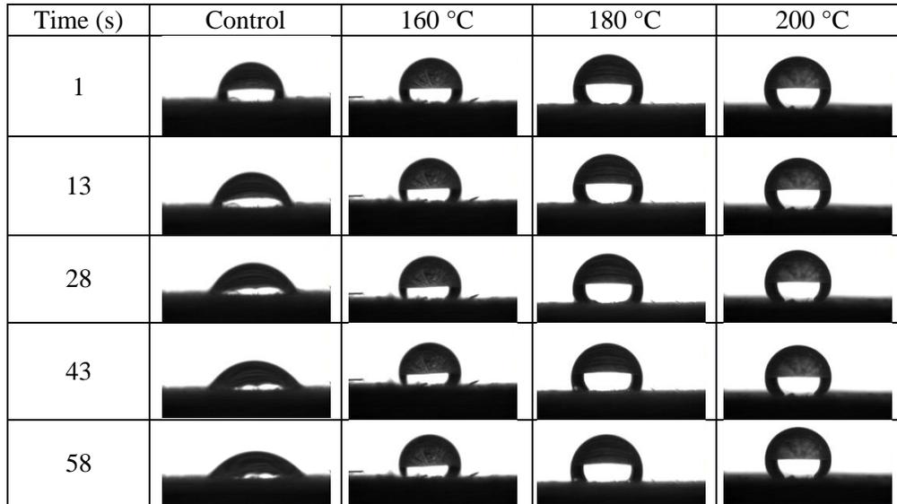
Fig. 6. Contact angles of royal paulownia before and after heat treatment
